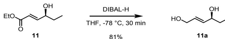
To a cooled (-78 °C) solution of known ester<sup>2</sup> **11** (16.5 g, 104.0 mmol) in THF (500 mL) was added DIBAL-H (1 M in toluene, 208 mL, 208.0 mmol). The mixture was stirred for 30 min at the same temperature, quenched with saturated Rochelle's solution (500 mL), extracted with *i*PrOH/CHCl<sub>3</sub> (1:4).
