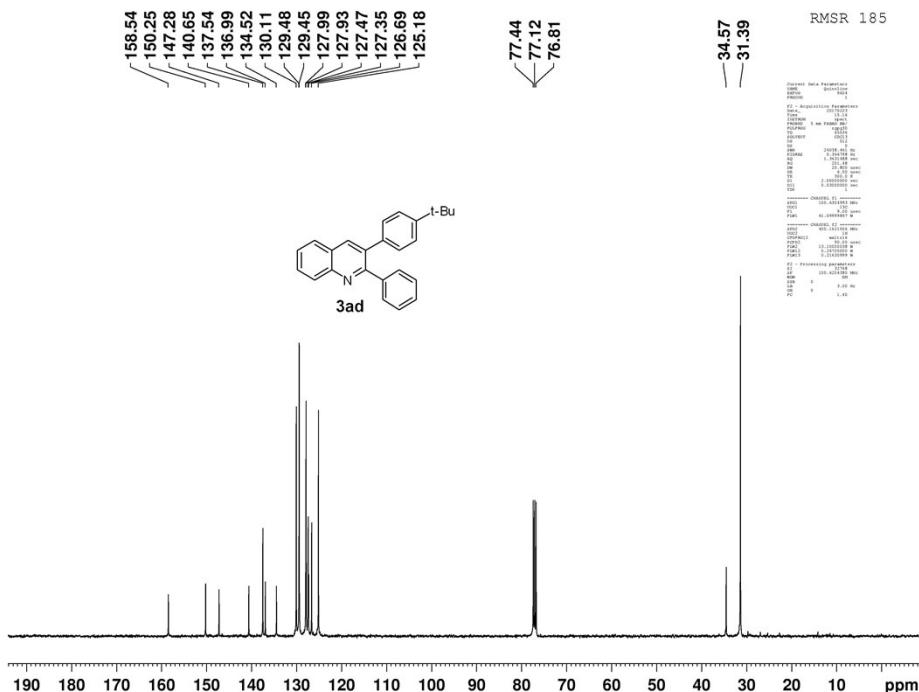
Fig. S8  $^{13}\text{C}$  NMR of 3ad
