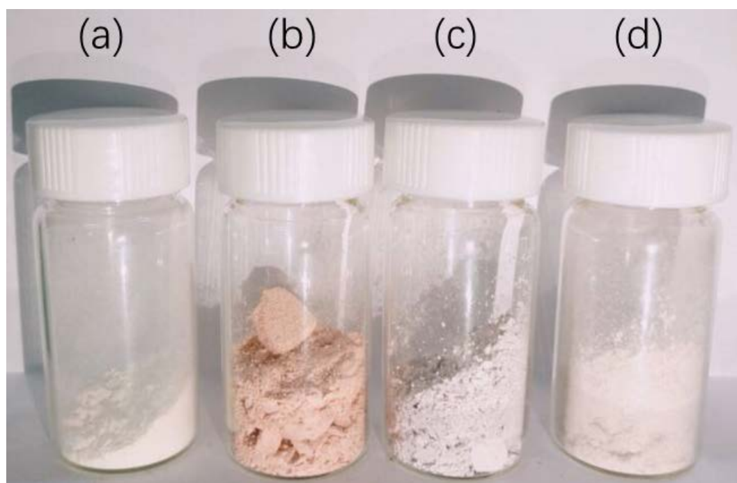
Fig. S2 Photos of as-synthesized \text{C}_5\text{H}_7\text{LiO}_2 (a), \text{LiCo}(\text{acac})_3 (b), \text{LiNi}_{0.8}\text{Co}_{0.2}(\text{acac})_3 (c), and \text{LiNi}_{0.5}\text{Co}_{0.2}\text{Mn}_{0.2}(\text{acac})_3 (d).
