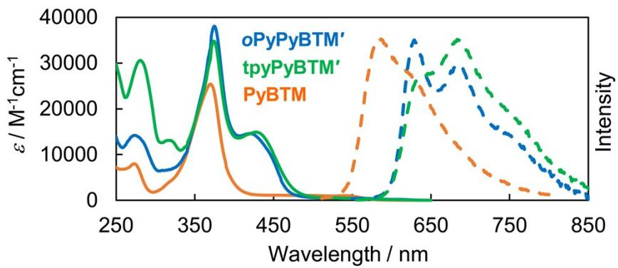
**Fig. S2** Absorption and emission spectra of PyBTM (orange line), *o*PyPyBTM' (blue line), and tpyPyBTM' (green line) in dichloromethane.
