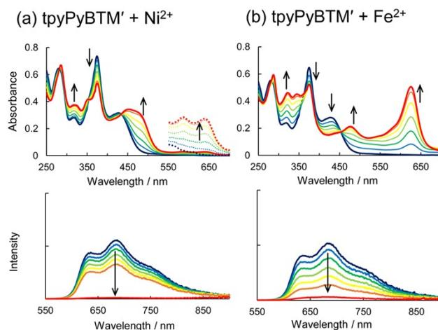
**Fig. S3** Changes in the absorption and emission spectra of (a) tpyPyBTM' during titration with Ni<sup>II</sup>(AcO)<sub>2</sub>, and (b) tpyPyBTM' during titration with Fe<sup>II</sup>SO<sub>4</sub> in dichloromethane. (navy: original spectra.; blue: 0.2 eq.; green: 0.4 eq.; yellow green: 0.6 eq.; yellow: 0.8 eq.; orange: 1.0 eq.; red: final spectra). In all emission spectra, excitation light was irradiated at the longest wavelength isosbestic point.
