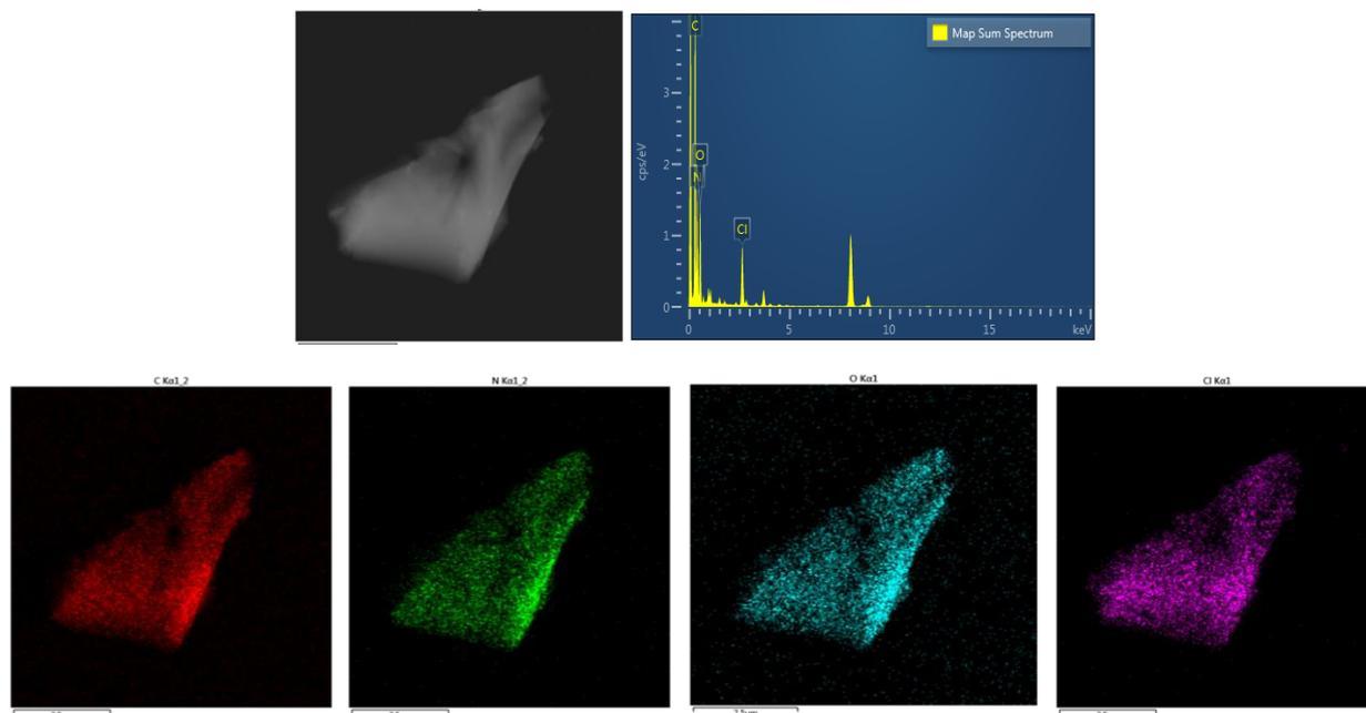
**Fig. S9** The element distribution mapping images of **SOF-CHO**, confirming the compositions of the C, N, O and Cl elements by the energy-dispersive X-ray spectroscopy.
