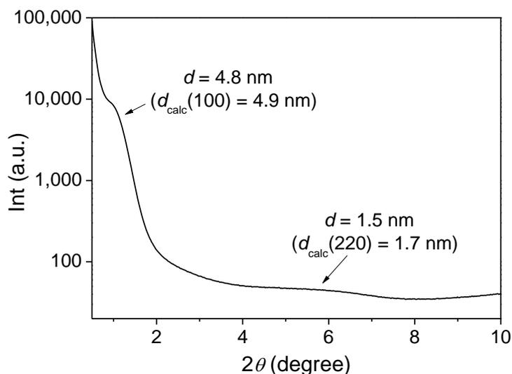
**Fig. S13** XRD of solid-state SOF-CH=N-[Ru(BPY)<sub>3</sub>] after 10 runs of the catalysis reaction.
