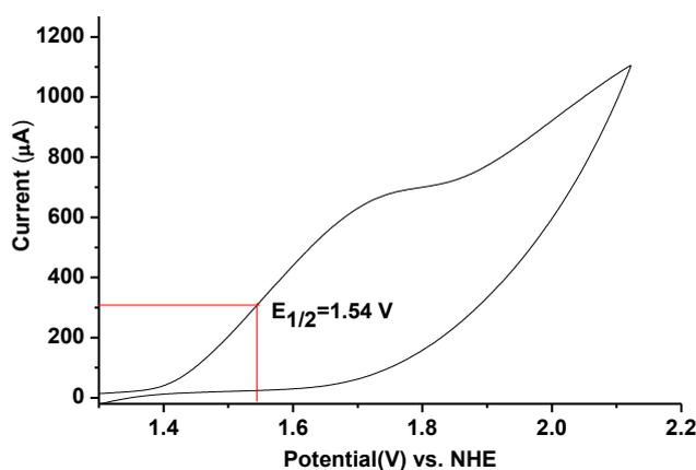
**Fig. S12** Cyclic voltammetry of **2** (0.2 mM) in the aqueous solution of KCl (100 mM) with a scan rate of 100 mV/s. Working, reference, and counter electrodes are platinum disk electrode, Ag/AgCl, and Pt, respectively.
