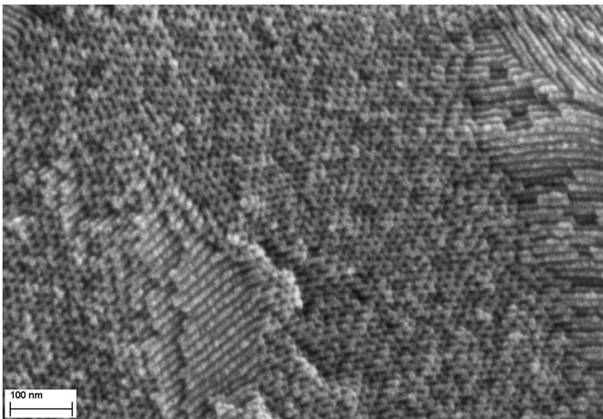
**Figure S14.** SEM recording of mesoporous carbon based on  $\text{PPO}_{66}\text{-PEO}_{180}\text{-PPO}_{66}$  as structure-directing agent.
