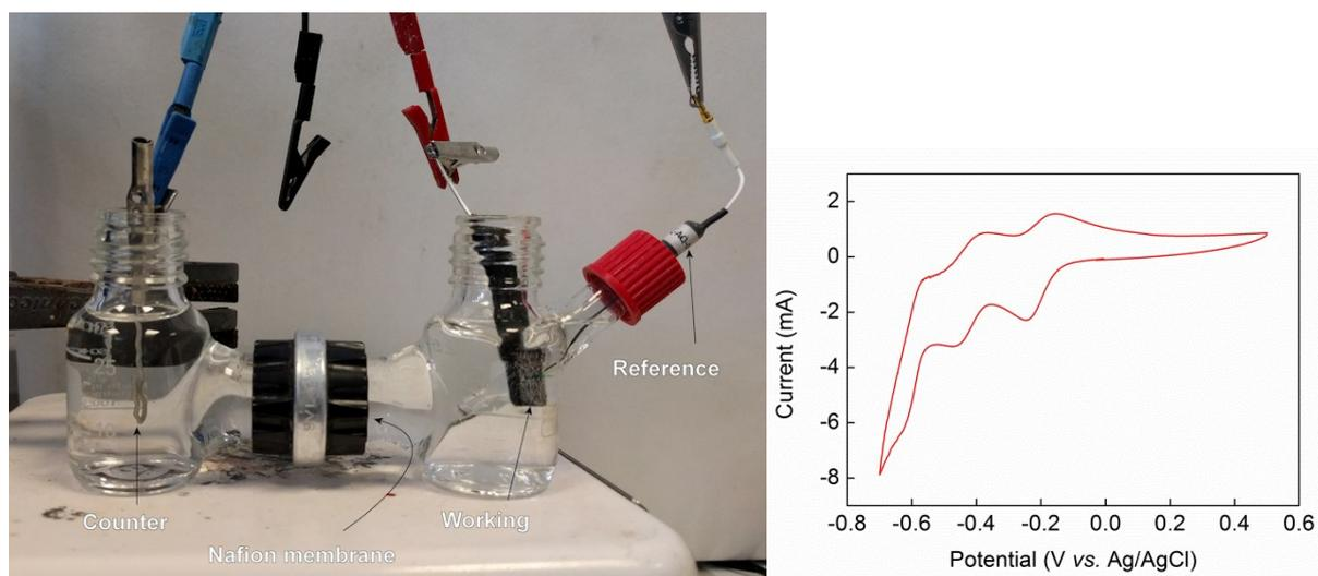
**Figure S1, Left:** H-cell, with a working (carbon felt) and reference electrode (Ag/AgCl) separated by a Nafion membrane from the counter electrode (Pt wire). **Right:** a cyclic voltammogram under Ar and at room temperature of a 0.5 M STA solution in water (pH 0.5) at a glassy carbon working electrode (area =  $0.071 \text{ cm}^2$ ) and a scan rate of 100 mV/s. A Pt-mesh counter electrode and an Ag/AgCl reference electrode were used.
