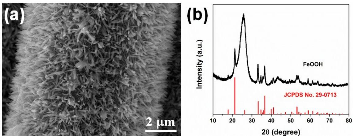
Figure S1. (a) FESEM image and (b) XRD patterns of FeOOH nanorod arrays.
