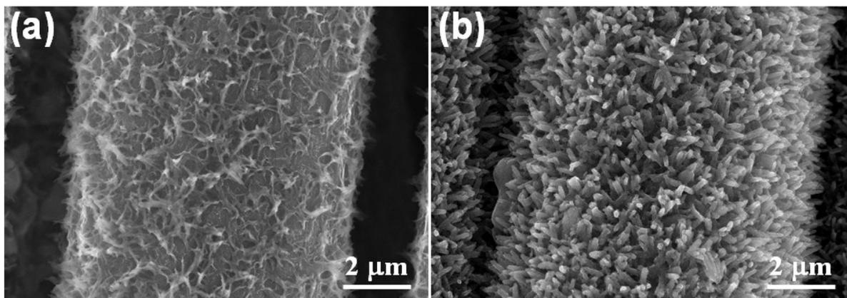
Figure S6. FESEM images of (a) FeP and (b) FeP/PEDOT nanorod arrays after cycling test.
