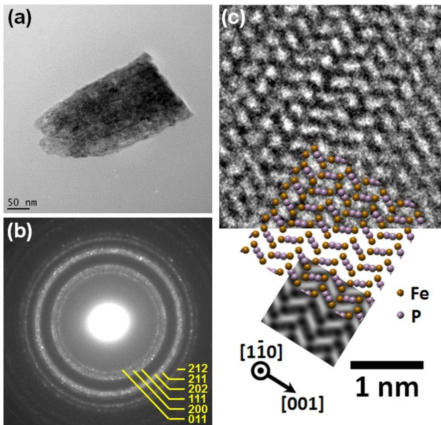
Figure S2. (a) TEM image, (b) SAED, and (c) HRTEM of FeP nanorod.
