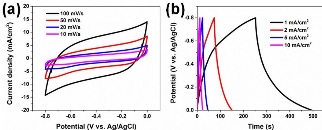
Figure S3. (a) CV curves of FeP electrode collected at scan rates from 10 to 100 mV/s. (b) Galvanostatic charge/discharge curves of FeP electrode at current densities from 1 to 10 mA/cm<sup>2</sup>.
