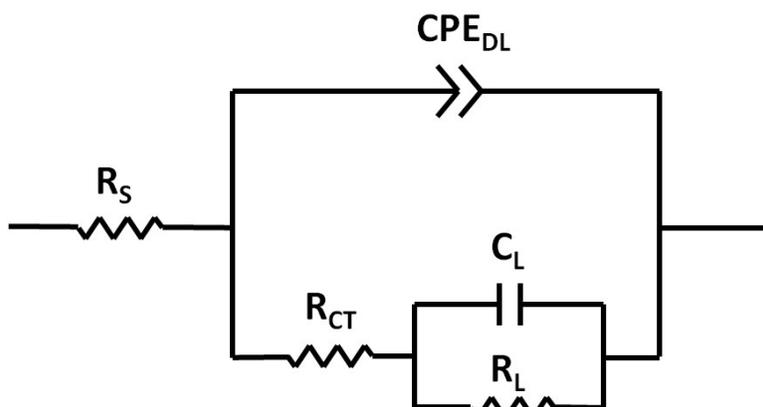
Figure S5. The equivalent circuit for the electrochemical impedance spectra.
