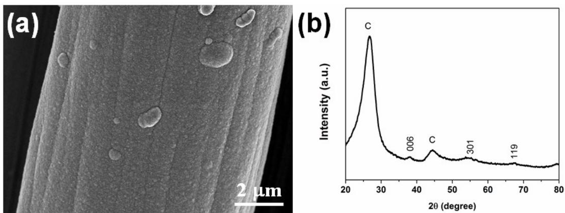
Figure S7. (a) FESEM image and (b) XRD patterns of MnO<sub>2</sub> electrode.
