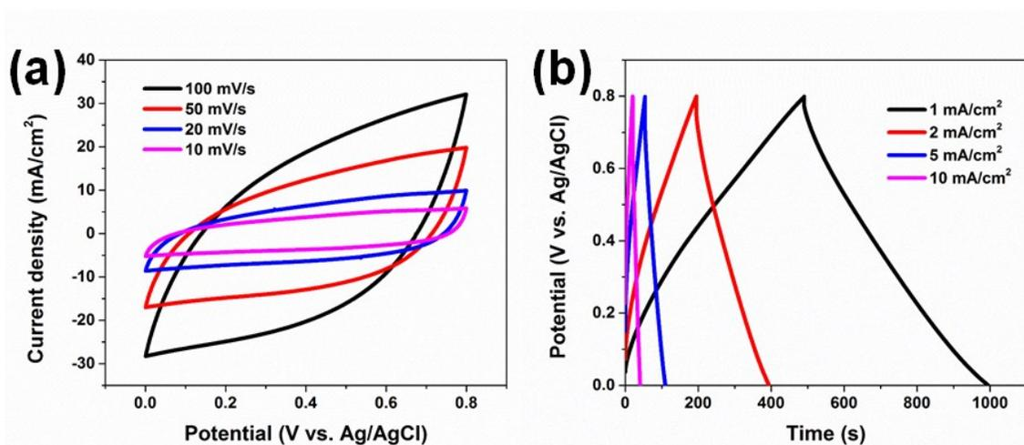
Figure S8. (a) CV curves of the MnO<sub>2</sub> electrode collected at scan rates from 10 to 100 mV/s. (b) Galvanostatic charge/discharge curves of the MnO<sub>2</sub> electrode at current densities from 1 to 10 mA/cm<sup>2</sup>.
