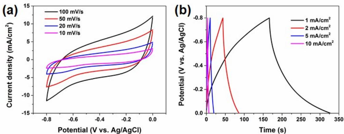
Figure S4. (a) CV curves of pure PEDOT collected at scan rates from 10 to 100 mV/s. (b) Galvanostatic charge/discharge curves of pure PEDOT at current densities from 1 to 10 mA/cm<sup>2</sup>.
