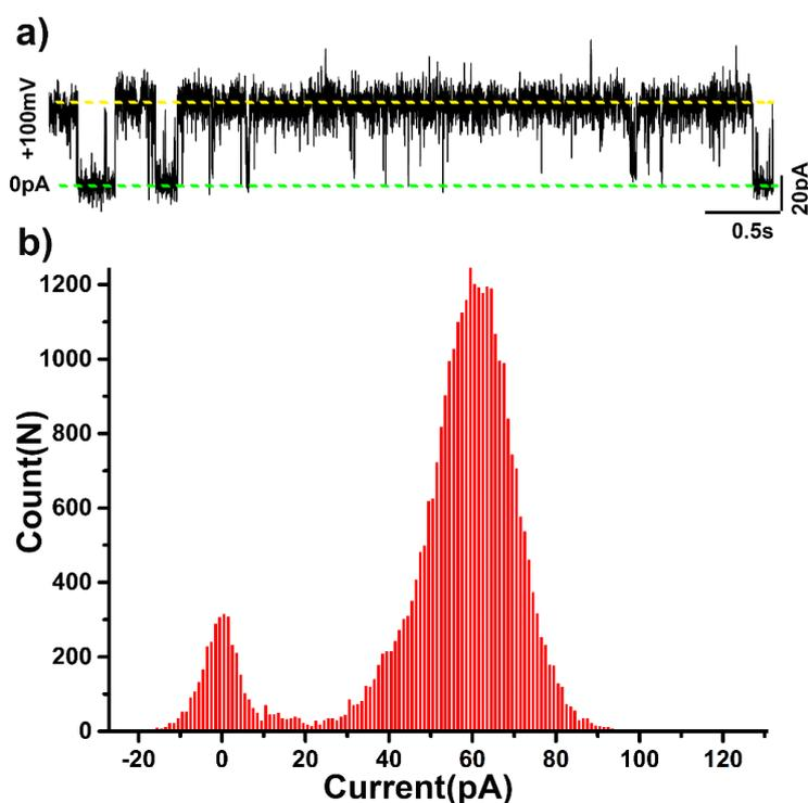
**Figure S8** Typical single-channel current recording a) and a histogram of the currents
