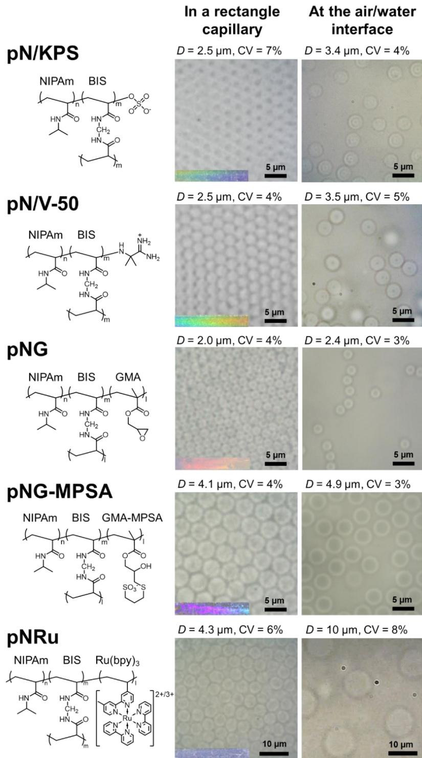
**Figure S1.** Optical microscopy images of different microgels. Inset photographs show colloidal crystals composed of each microgel. The microgels were observed in a rectangle capillary at high concentration (left column) and at the air/water interface (right column) of the dispersion droplets ( $N = 30$ ). From these images, it is clear that these microgels are uniform, and that the applied synthetic method should be applicable to various pNIPAm-based microgels.
