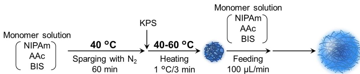
**Scheme S1.** pNA core-shell microgels prepared via a modified aqueous precipitation polymerization.
