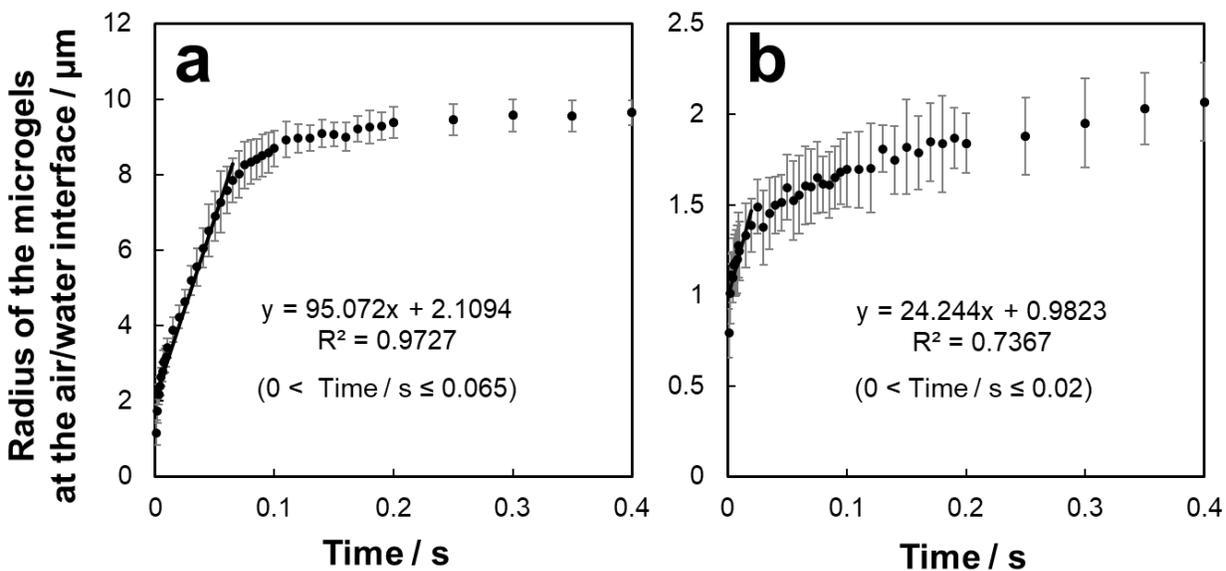
**Figure S3.** Radius of (a) pNA(1.4) and (b) pNA(2.7) microgels as a function of time at the air/water interface, which were calculated from the diameter (**Figure 2**).
