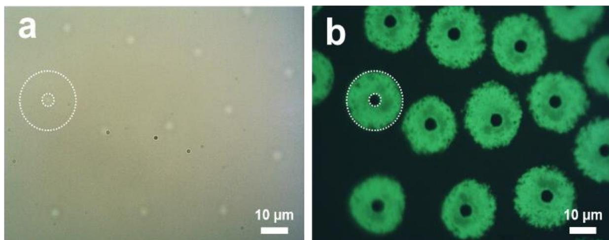
**Figure S2.** (a) Optical and (b) fluorescence microscopy images of the same pNA microgels after labelling with R6G dye molecules. The same area was observed at the air/water interface of the dispersion droplet at pH = 7 and 25 °C. The white dotted lines indicate the core part and the surface of an individual microgel.
