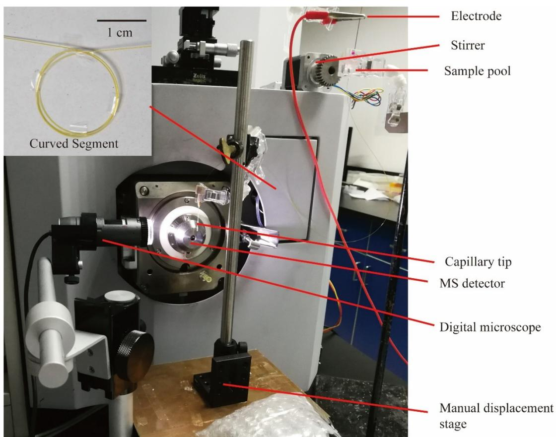
**Fig. S5** Photograph of the single-cell operation system. The device consists of a platinum electrode connected to the laboratory-made high-voltage power supply, video capture device (a digital microscope focused on the capillary tip showing the cell condition in the capillary and the Taylor cone), a magneton and stirrer to induce homogeneous cell suspension, the specially immobilized capillary a MS detector.
