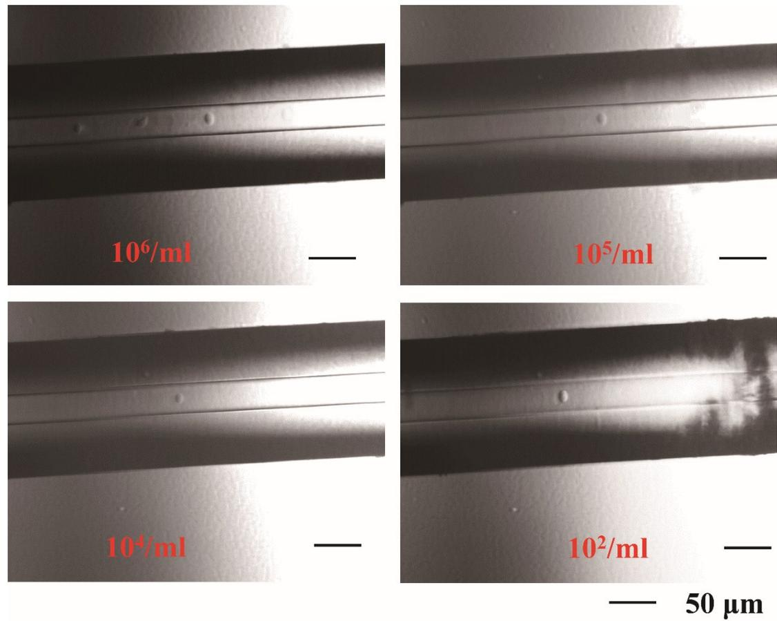
**Fig. S1** Cells in cell suspension observed near the outlet of capillary. Different concentrations from  $10^2$ - $10^5$  /ml are proved to be suitable for this device to separate single-cells.
