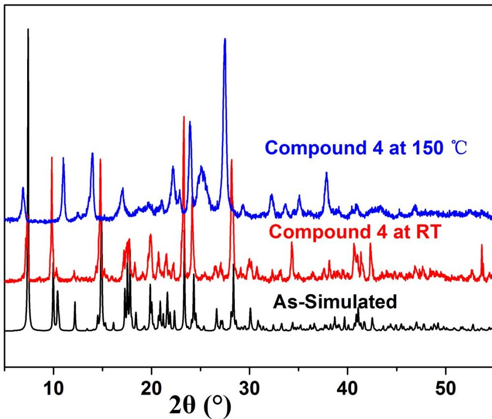
**Fig. S8** The PXRD patterns of **4** at room temperature and 150 °C.
