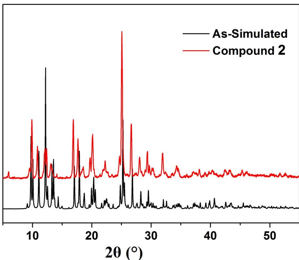
**Fig. S6** The PXRD patterns of **2** at room temperature.
