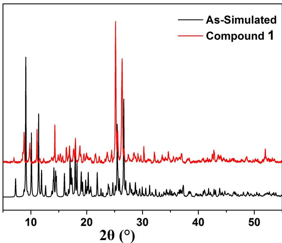
**Fig. S5** The Powder X-ray diffraction (PXRD) patterns of **1** at room temperature.
