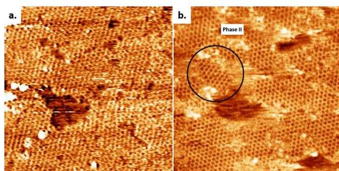
Figure S1. **(a)** STM image of COF-1 synthesized in 1,2,4-trichlorobenzene (TCB), collected at the air/solid interface. Image width: 60 nm. Scanning conditions:  $V = -1000$  mV,  $I = 100$  pA. **(b)** STM image of COF-1 synthesized in heptanoic acid, collected at the interface of heptanoic acid and HOPG. A small domain of Phase II is marked by black circle. Image width: 60 nm. Scanning conditions:  $V = -800$  mV,  $I = 100$  pA.
