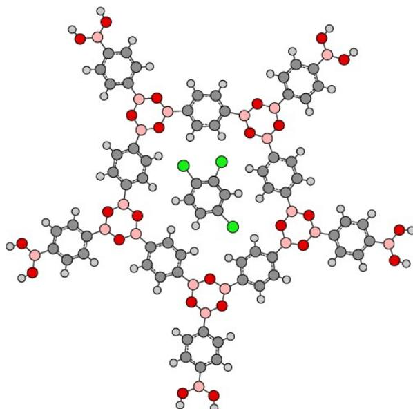
Figure S3. Indicative geometry for TCB in pentagonal pore. All H...H distances between hydrogens on the TCB molecule and hydrogens on the COF-1 pore are below 2 vdW radii for hydrogen ( $2r_{\text{H}}=2.4 \text{ \AA}$ ),<sup>[1]</sup> suggesting that the TCB molecule cannot be accommodated in a planar adsorption geometry in the pentagonal pore.
