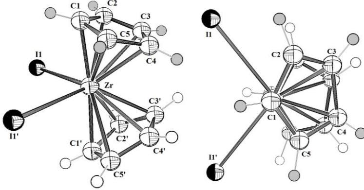
**Figure S20.** ORTEP diagram, drawn with 50% probability ellipsoids, showing the atomic labelling scheme for IDCPZR ( $\text{Cp}_2\text{ZrI}_2$ ).
