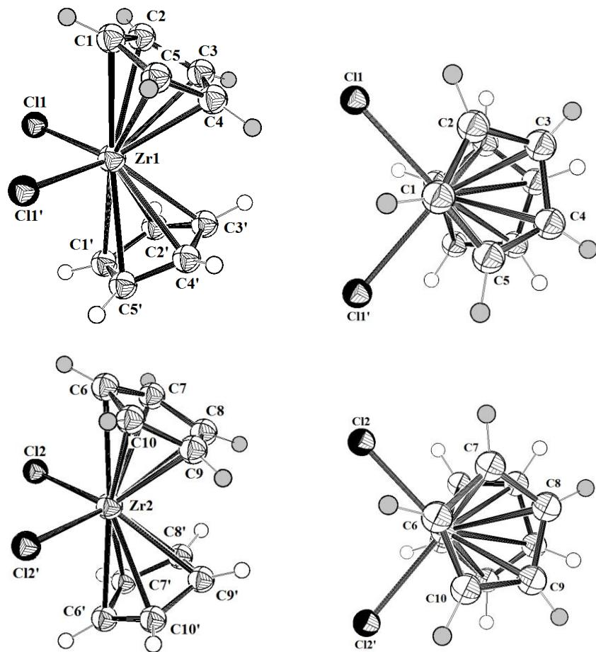
**Figure S3.** ORTEP diagram, drawn with 50% probability ellipsoids, showing the atomic labelling scheme for the two types of molecules of CPDCZR04 ( $\text{Cp}_2\text{ZrCl}_2$ ) (type A molecules on top, type B below).
