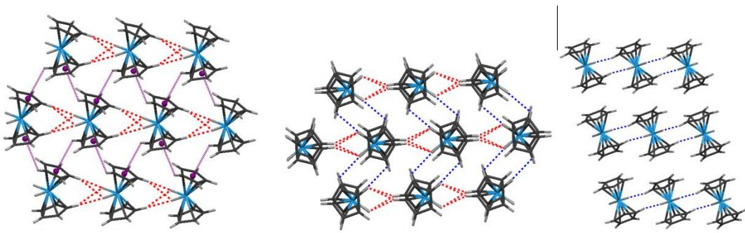
**Figure S23** – Supramolecular arrangement of  $\text{Cp}_2\text{WH}_2$ . Planes of chains formed by  $\text{C}-\text{H}\cdots\text{H}^-$  interactions (in red) and  $\text{C}-\text{H}\cdots\pi$  contacts (in purple) (left). Interaction between these planes by  $\text{C}-\text{H}\cdots\text{H}^-$  interactions (in blue): top (centre) and front (right) views.
