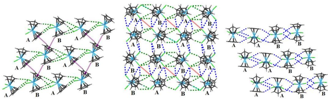
**Figure S6 –** Supramolecular arrangement of  $\text{Cp}_2\text{HfCl}_2$ . Planes of chains formed by  $\text{C}-\text{H}\cdots\text{Cl}$  interactions (in green) and  $\text{C}-\text{H}\cdots\pi$  contacts (in purple) (left). Interaction between these planes by  $\text{C}-\text{H}\cdots\text{Cl}$  interactions (in blue) and  $\text{Cl}\cdots\text{Cl}$  interactions (in red): top (centre) and front (right) views.
