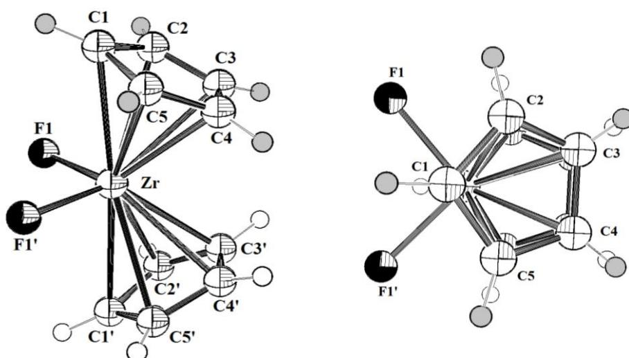
**Figure S1.** ORTEP diagram, drawn with 50% probability ellipsoids, showing the atomic labelling scheme for FDCPZR ( $\text{Cp}_2\text{ZrF}_2$ ). The molecule was labelled clockwise with the bonds that lay in the middle of the F-Zr-F angle designated as C(1)-H(1) and C(1')-H(1'). Halogen atoms have been coloured in black, hydrogen atoms of the upper ring in grey and all the atoms of the lower ring identified by a ' superscript.
