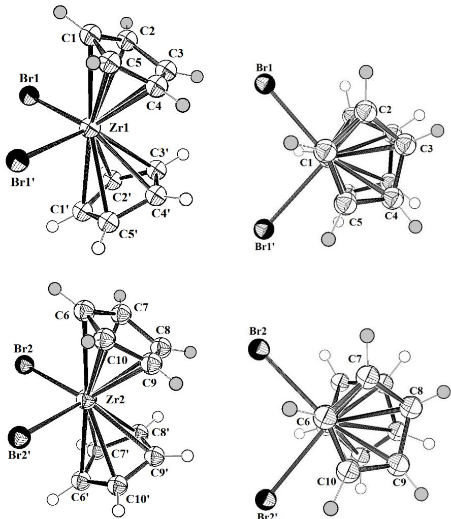
**Figure S16.** ORTEP diagram, drawn with 50% probability ellipsoids, showing the atomic labelling scheme for the two types of molecules of ZUJLOF ( $\text{Cp}_2\text{ZrBr}_2$ ) (type A molecules on top, type B below).
