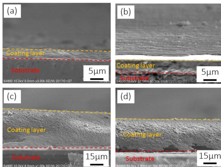
**Figure S1** Cross-sectional Field Emission-SEM (FE-SEM) images of the  $\text{Cu}_3(\text{BTC})_2$  coatings prepared at different EtOH:H<sub>2</sub>O volume ratio; (a) 1:0, (b) 5:2, (c) 1:1, (d) 2:5. Broken red and orange lines show the substrate/coating and coating/air interfaces, respectively. The thickness of the films was (a) 3.1, (b) 5.1, (c) 41.5 and (d) 37.1  $\mu\text{m}$ .
