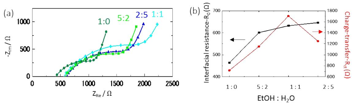
**Figure S4** (a) The electrochemical impedance spectra of the Cu<sub>3</sub>(BTC)<sub>2</sub> coatings on gold electrodes in the frequency range of 100 kHz to 10 mHz with an AC voltage amplitude of 10 mV in 0.1 M tetraoctylammonium tetrafluoroborate ([CH<sub>3</sub>(CH<sub>2</sub>)<sub>7</sub>]<sub>4</sub>N(BF<sub>4</sub>)). (b) Interfacial resistance  $R_0$  and charge-transfer- $R_{ct}$  calculated from the electrochemical impedance spectra.
