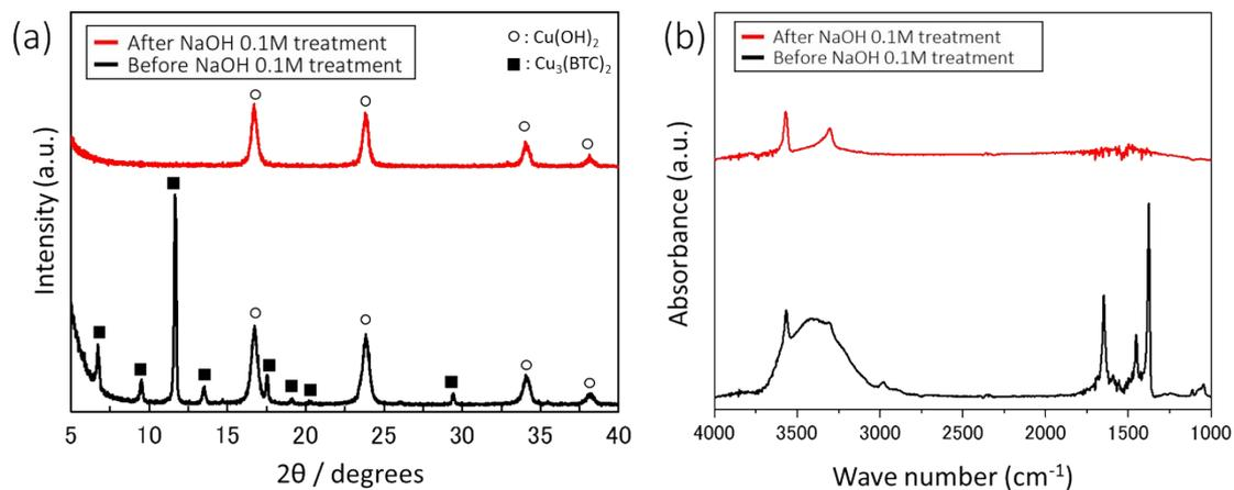
**Figure S6** (a) XRD patterns and (b) FTIR spectra of  $\text{Cu}_3(\text{BTC})_2$  MOF coating prepared at 1:1 before and after soaking into the NaOH electrolytic solution for electrocatalytic glucose oxidation.
