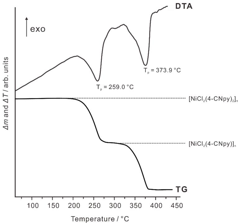
**Fig. S1** DTA/TG curves of  $[\text{NiCl}_2(4\text{-CNpy})_2]_n$  (**3a**). Weight of starting compounds: 31.92 mg, Heating rate: 5 K/min, N<sub>2</sub> atmosphere, Al<sub>2</sub>O<sub>3</sub> crucible, T<sub>p</sub>: peak temperature.
