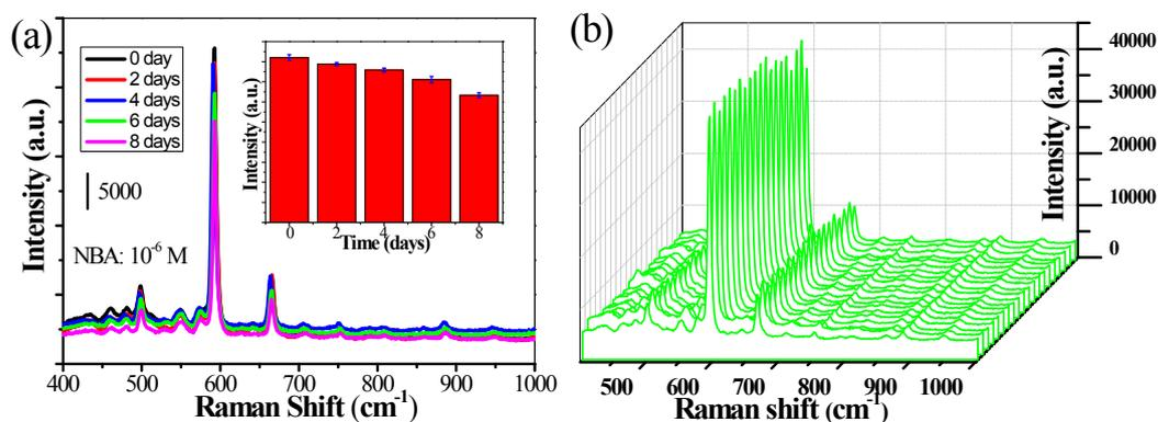
**Figure S5** (a) SERS spectra of following Au nanocages substrate storage at room temperature. Inset depicts the histogram of storage time and SERS intensity at 592  $\text{cm}^{-1}$ . (b) SERS spectra of NBA at 20 random points from different area of substrate.
