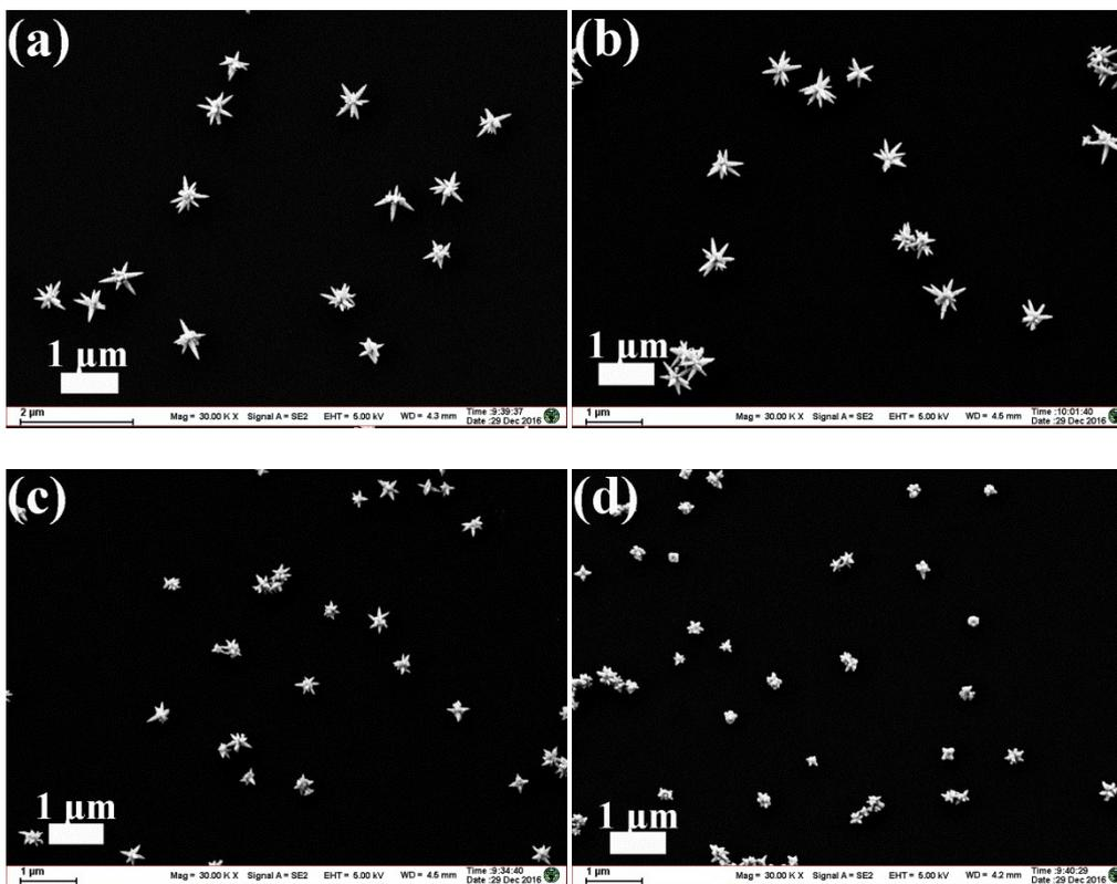
Figure S2 SEM images of as-prepared Ag nanoechinus by using different volumes of Ag seed solution: (a) 20 μL, (b) 40 μL, (c) 60 μL and (d) 100 μL.
