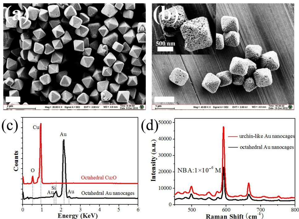
**Figure S6** SEM images of as-obtained (a) octahedral Cu<sub>2</sub>O, (b) octahedral Au nanocages. The bar is 1  $\mu\text{m}$ . (c) EDS analysis of the obtained octahedral Cu<sub>2</sub>O and Au nanocages. (d) A comparison in SERS activity of urchin-like Au nanocages and octahedral Au nanocages for the detection of NBA.
