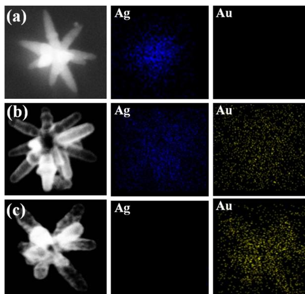
**Figure S3** Elemental mapping images of as-prepared (a) Ag nanoechinus, (b) Au-Ag alloy(adding 50 $\mu$ L H<sub>2</sub>AuCl<sub>4</sub>), (c) urchin-like Au nanocage.
