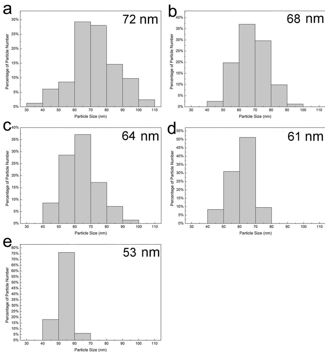
**Figure S3.** Size distribution of CuNPs synthesized from a 5 mM  $\text{CuSO}_4$ -based electrolyte with 10 mM  $\text{Na}_3\text{CA}$  for 1000 s at (a) -0.20 V, (b) -0.23 V, (c) -0.26 V, (d) -0.29 V, (e) -0.32 V vs.  $\text{Ag}|\text{AgCl}$ .
