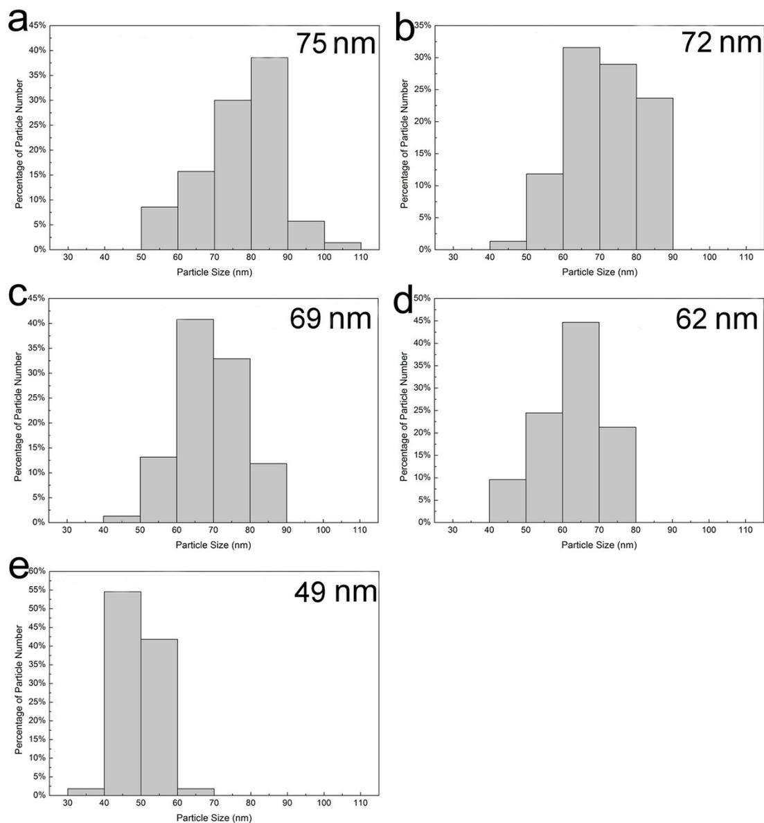
**Figure S2.** Size distribution of CuNPs synthesized from a 2 mM  $\text{CuSO}_4$ -based electrolyte with 5 mM  $\text{Na}_3\text{CA}$  for 1000 s at (a) -0.23 V, (b) -0.26 V, (c) -0.29 V, (d) -0.32 V, (e) -0.35 V vs.  $\text{Ag}|\text{AgCl}$ .
