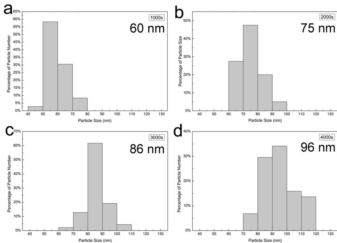
**Figure S4.** Size distribution of CuNPs synthesized from a 2 mM CuSO<sub>4</sub>-based electrolyte with 10 mM Na<sub>3</sub>CA at -0.32 V vs. Ag|AgCl for (a) 1000 s, (b) 2000 s, (c) 3000 s, (4) 4000 s.
