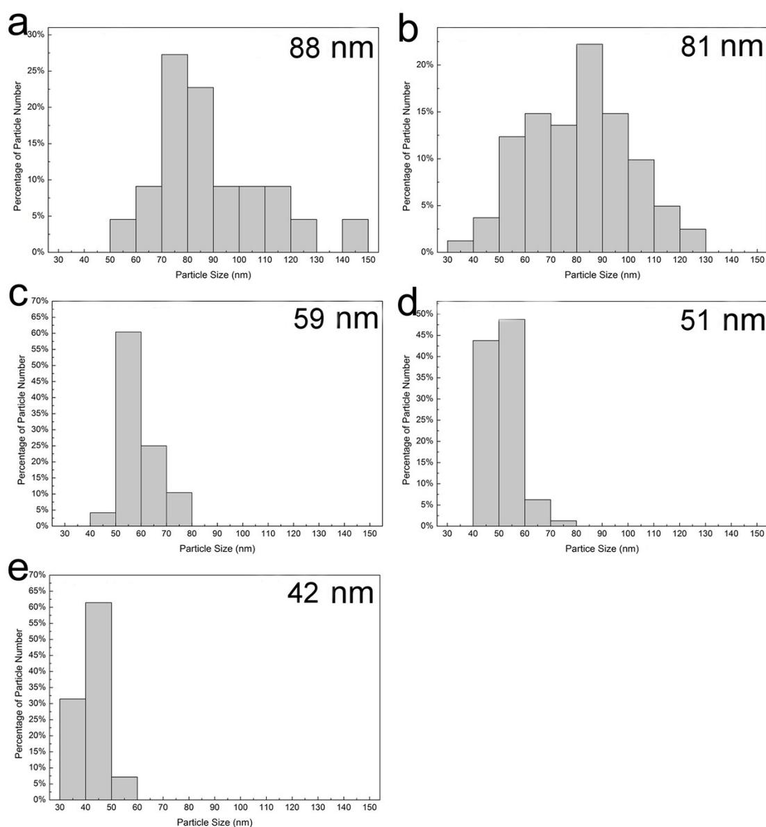
**Figure S1.** Size distribution of CuNPs synthesized from a 2 mM  $\text{CuSO}_4$ -based electrolyte with 10 mM  $\text{Na}_3\text{CA}$  for 1000 s at (a) -0.26 V, (b) -0.29 V, (c) -0.32 V, (d) -0.35 V, (e) -0.38 V vs.  $\text{Ag}|\text{AgCl}$ .
