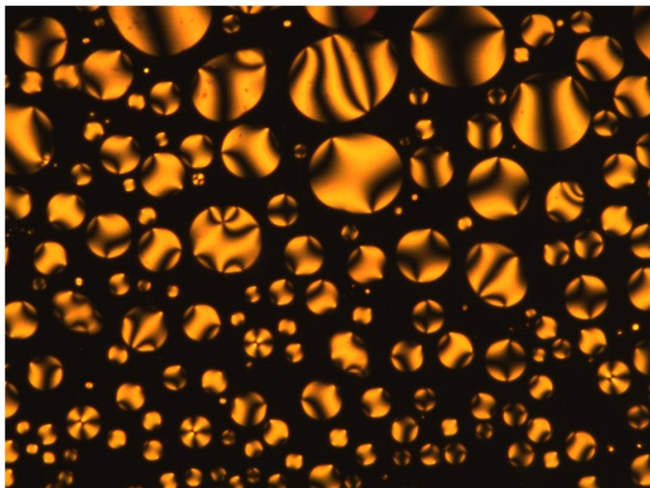
**Fig. S12** Optical texture of the nematic phase of 3-A6 at  $115\text{ }^{\circ}\text{C}$  on cooling from isotropic.
