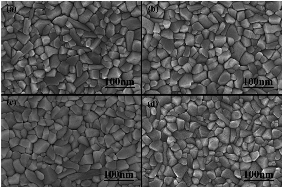
**Fig. S4** Top morphology of different samples after 500°C annealing (a)  $\text{Na}_x\text{WO}_3/\text{BK7}$ , (b)  $\text{WO}_{3-x}/\text{SiO}_2$ , (c)  $\text{Na}_2\text{W}_2\text{O}_7/\text{BK7}$ , (d)  $\text{WO}_3/\text{SiO}_2$
