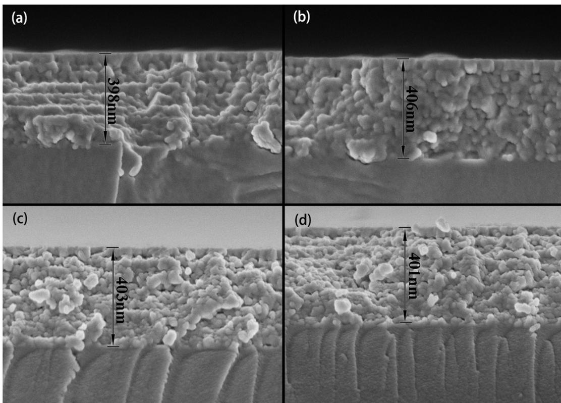
**Fig. S5** Cross morphology of different samples after 500°C annealing (a)  $\text{Na}_x\text{WO}_3/\text{BK7}$ , (b)  $\text{WO}_{3-x}/\text{SiO}_2$ , (c)  $\text{Na}_2\text{W}_2\text{O}_7/\text{BK7}$ , (d)  $\text{WO}_3/\text{SiO}_2$
