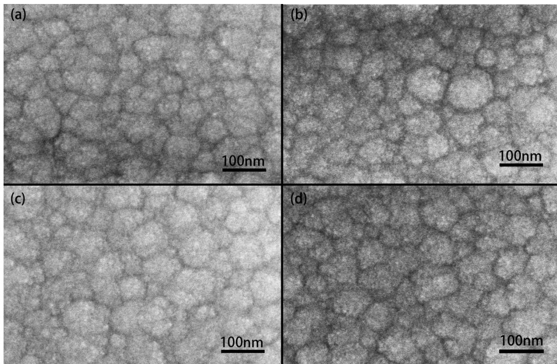
Fig. S3 Top morphology of different samples before annealing (a) WO<sub>3-x</sub>/BK7, (b) WO<sub>3-x</sub>/SiO<sub>2</sub>, (c) WO<sub>3</sub>/BK7, (d) WO<sub>3</sub>/SiO<sub>2</sub>
