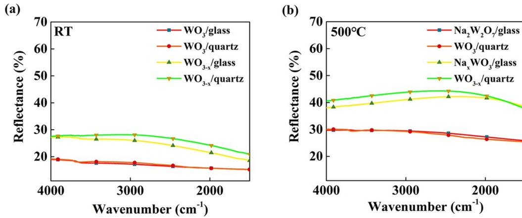
Fig. S2 FTIR spectra of (a) as-prepared samples and Na<sub>x</sub>WO<sub>3</sub> film (b) annealed at 500°C.
