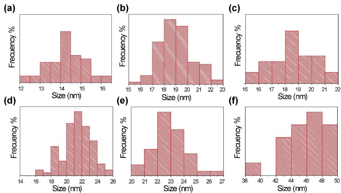
**Figure S2.** The particle size distribution of  $\text{NaGdF}_4@\text{NaGdF}_4:\text{Yb/Tm}$  core with different Na and RE precursor: (a) CSUC-1#, (b) CSUC-2#, (c) CSUC-3#, (d) CSUC-4#, (e) CSUC-5# and (f) CSUC-6#.
