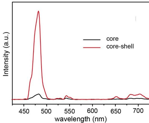
**Figure S3.** The emission spectrum of core-shell UCNPs (CSUC-6#) with its core(UC-6#).
