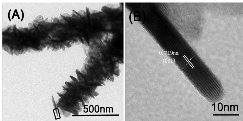
**Fig.S4** the TEM and HRTEM images of BiOCl-110 sample.
