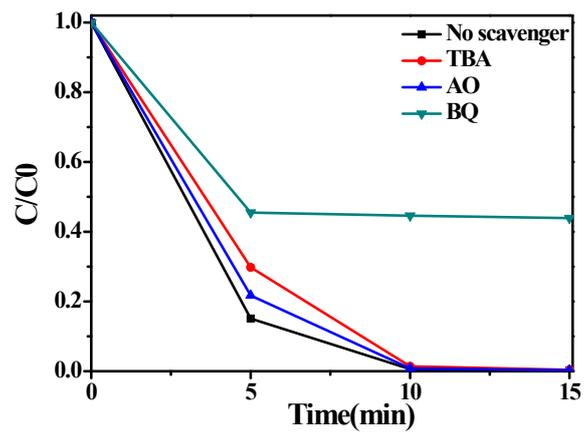
**Fig. S8** Active species trapping experiments during the photocatalytic degradation to MO (20 mg/L) under solar light irradiation using BiOBr-110 as photocatalyst.
