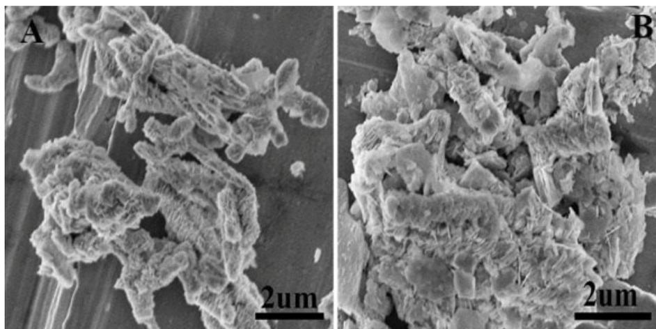
**Fig. S5** SEM images of BiOBr-110 obtained at different concentration of reactants (A) 0.5 mmol, and (B) 2 mmol.
