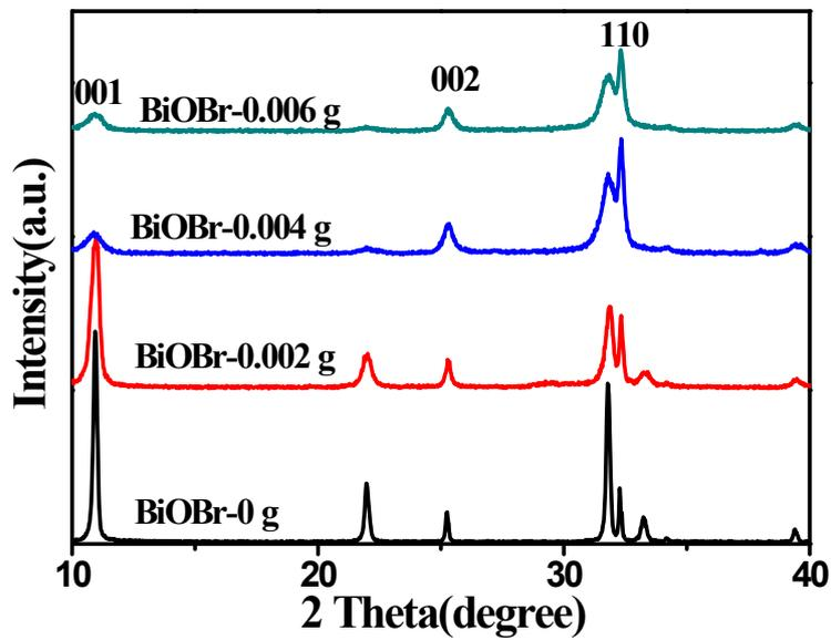
**Fig. S2** The XRD patterns of the obtained BiOBr samples with different concentration of glucose (0, 0.002, 0.004 and 0.006g).
