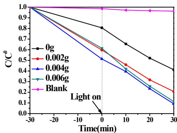
**Fig. S6** the degradation curve of MO using BiOBr samples obtained at different concentration of glucose as photocatalyst under visible light irradiation.
