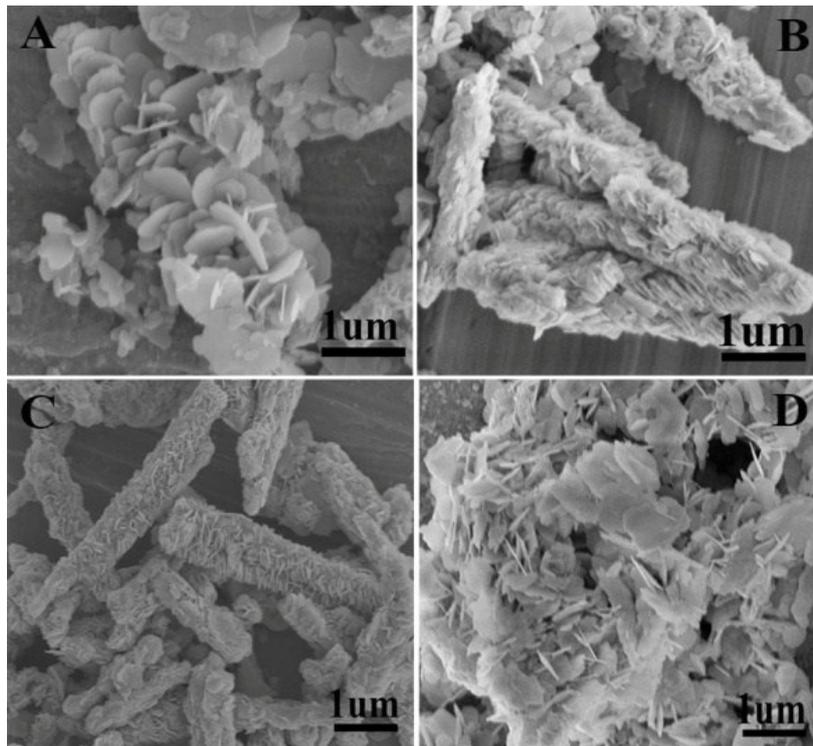
**Fig. S3** SEM images of BiOBr at 160° C for different reaction time using 0.004g of glucose as surfactant, (A) 2 h, (b) 6 h, (c) 12 h, (d) 24 h.
