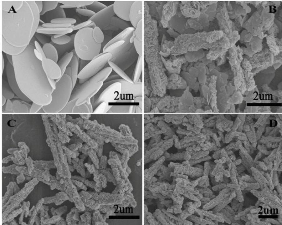
**Fig. S1** SEM images of the obtained BiOBr with the different concentration of glucose, (A) 0 g, (B) 0.002 g, (C) 0.004 g and (D) 0.006 g.
