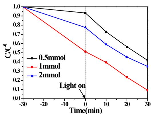
**Fig. S7** the degradation curve of MO using BiOBr samples obtained at different concentration of reactant as photocatalysts under visible light irradiation
