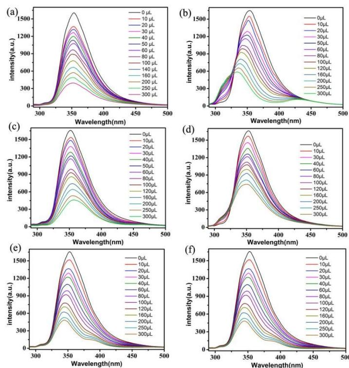
Fig. S6 Effect on the emission spectra of **3** dispersed in DMSO with increasing addition of a nitrobenzene derivative solution (a. NT; b. NA; c. NP; d. 1,3-DNB; e. 2,4-DNT; f. PA).
