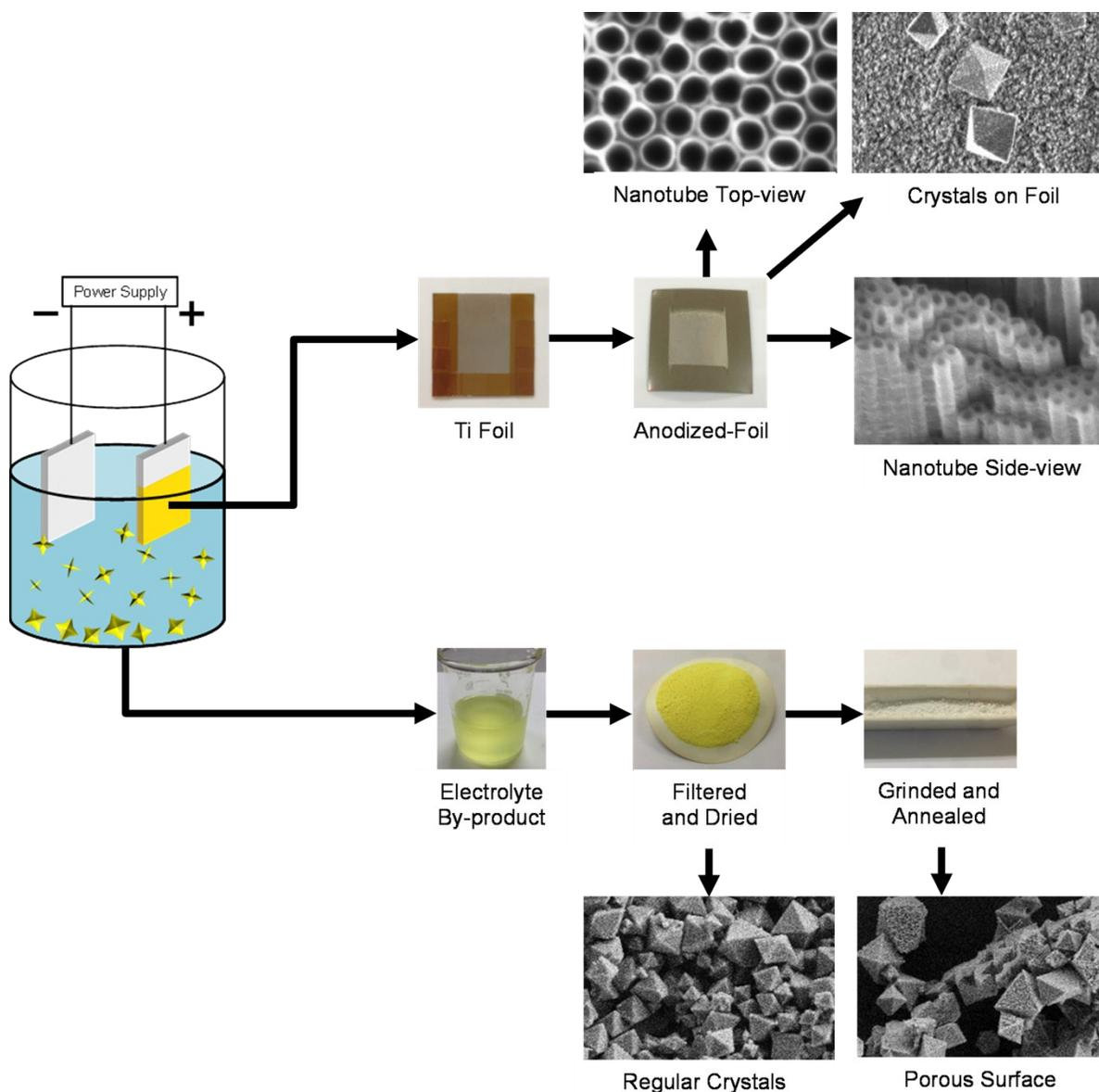
**ESI Figure 1| Anodization produces Titania Nanotube (TNT) on foil surface and generate unwanted electrolyte (by-product). Nanotube and octahedral crystals are found on foil surface. The yellowish electrolyte is filtered and dried. After annealing, the yellowish precipitate turns into whitish compounds.**
