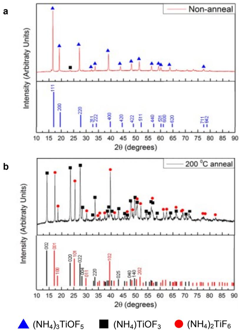
**ESI Figure 6** | XRD diffractograms with  $hkl$  information. a, Pre-anneal yellowish powder fits well with  $(\text{NH}_4)_3\text{TiOF}_5$ . b, Post-anneal white powder show the presence of  $(\text{NH}_4)\text{TiOF}_3$  and  $(\text{NH}_4)_2\text{TiF}_6$ .
