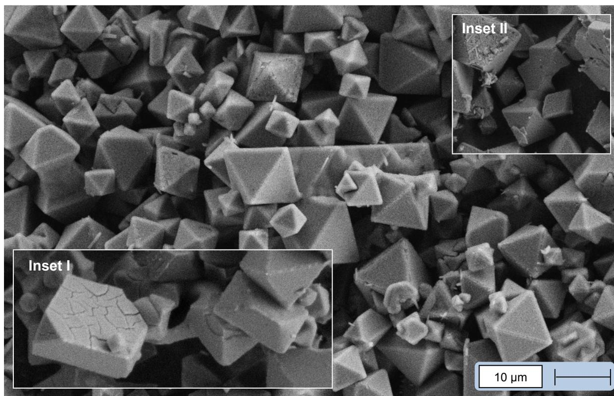
**ESI Figure 2** | FESEM overview on the pre-annealed precipitate. **Inset I**, (Left) Truncated structure (Right) Elongated structure. **Inset II**, Stacking of octahedron crystals at (001) and (111) planes.
