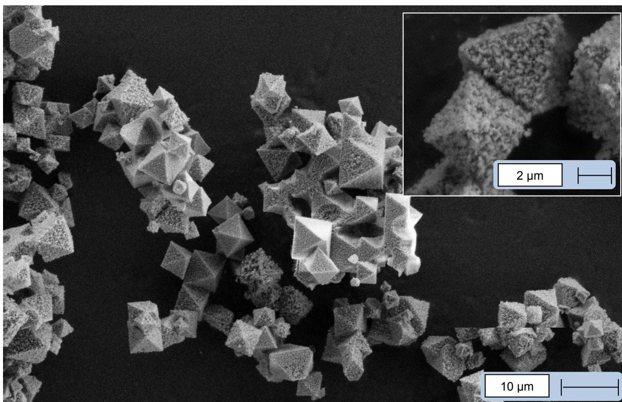
**ESI Figure 4|** FESEM overview on the post-annealed precipitate. **Inset,** Magnified view on post-annealed octahedral crystal. The crystal retains its octahedron shape with roughen surface due to decomposition of  $(\text{NH}_4)_3\text{TiOF}_5$  compounds.
