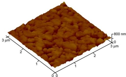
Nanoparticle substrate:  $R_q = 6.7 \pm 0.4$  nm
