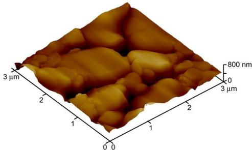
Microcrystal substrate:  $R_q = 1.9 \pm 0.1$  nm
