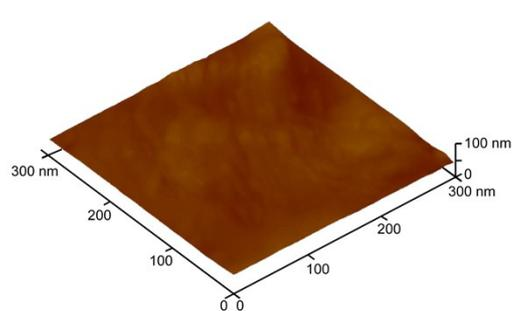
Nanoparticle substrate:  $R_q = 38 \pm 4$  nm
