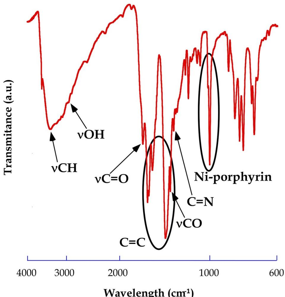
**Figure S1.** IR Spectra of compound 1.
