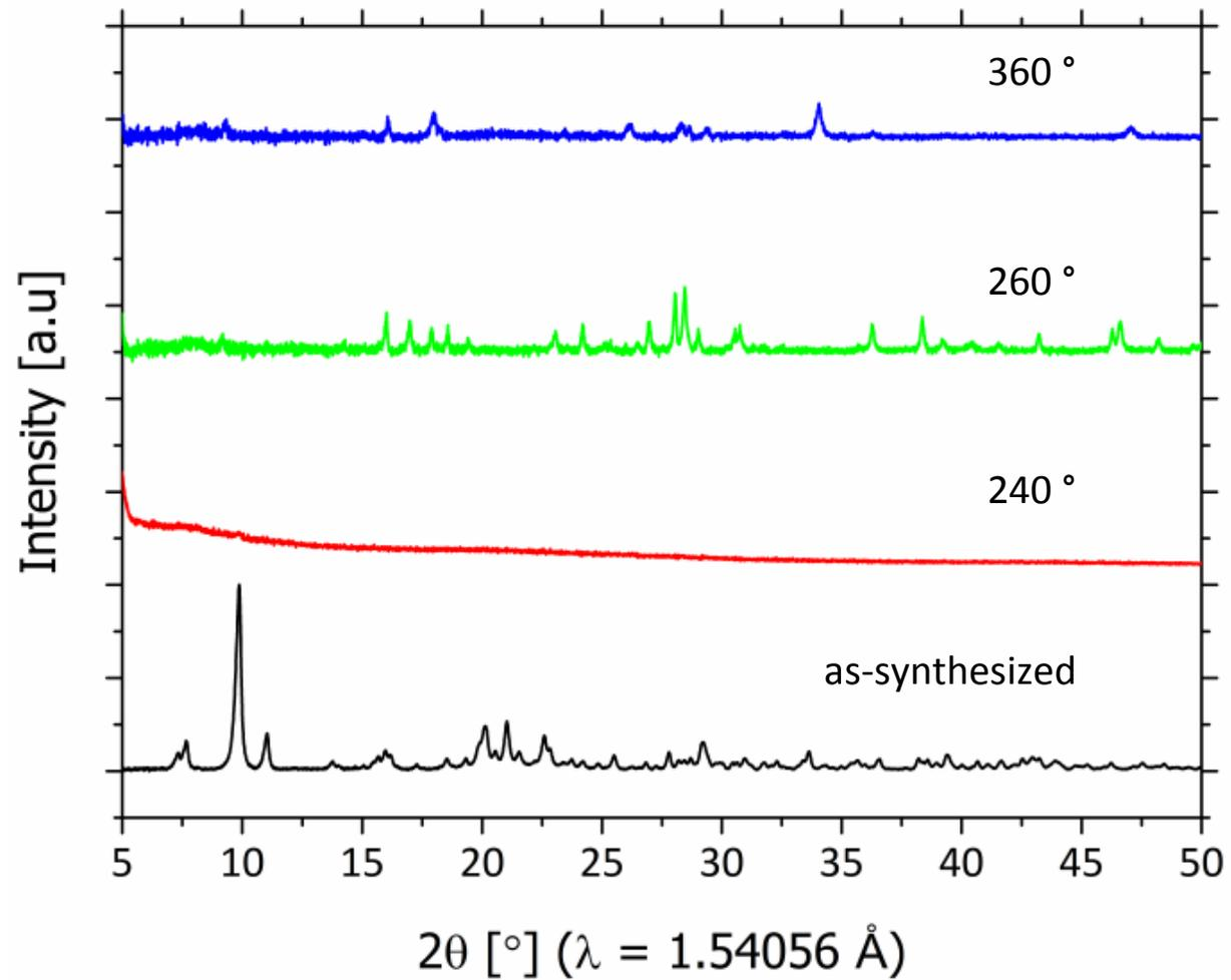
**Figure S6.** PXRD patterns of the compound  $[\text{Ca}(\text{mBDC})(\text{H}_2\text{O})_{3.4}]$  (**2**) as-synthesized (black PXRD patterns) and after the thermal post-treatments at different temperatures (red, green, and blue PXRD patterns)
