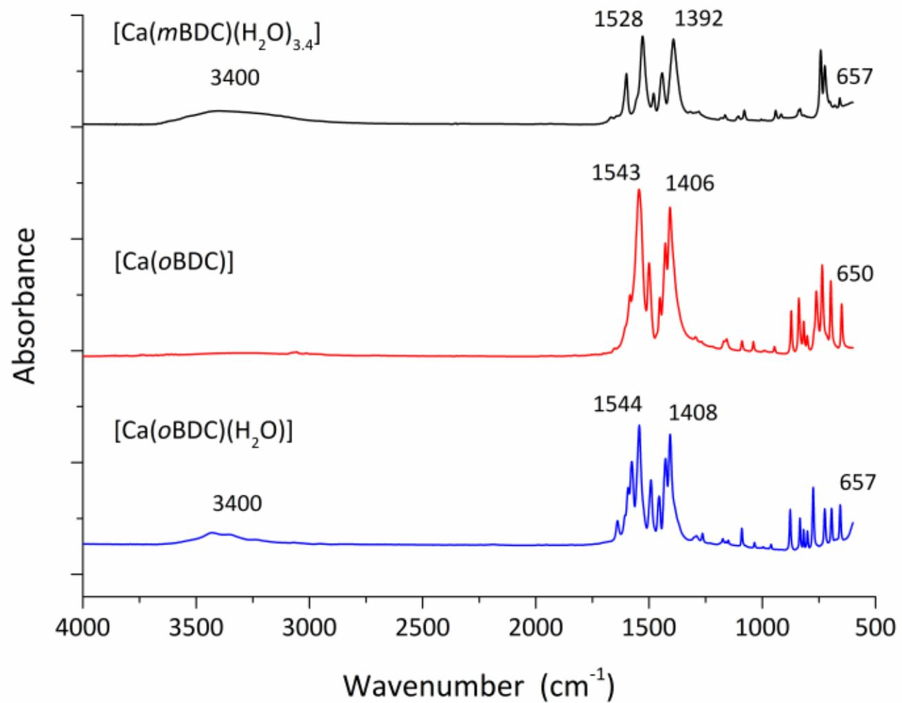
**Figure S7.** The ATR-IR spectra of compound **1** (blue spectrum), compound (**1-H<sub>2</sub>O**) (red spectrum), and compound **2** (black spectrum).
