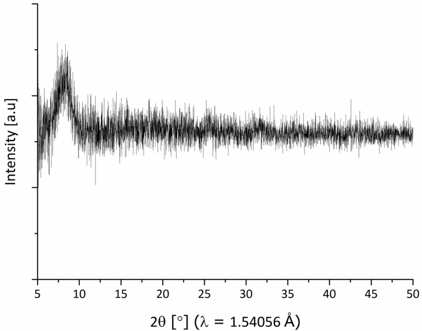
**Figure S2.** PXRD pattern of the amorphous product obtained by milling  $\text{H}_2\text{mBDC}$  and  $\text{Ca}(\text{OH})_2$  without adding water. Milling time = 4h. The molar ratio between organic and inorganic reactants was 1:1.
