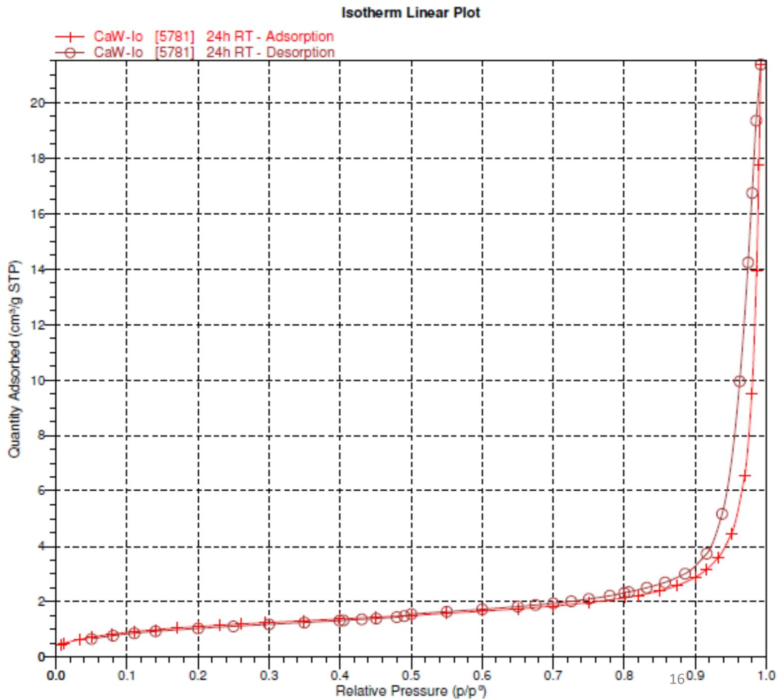
**Figure S9.** Isotherm curves of the compound [Ca(oBDC)] (1-H<sub>2</sub>O). Adsorption (crosses) and desorption pore volume (circles) isotherm for nitrogen at room temperature
