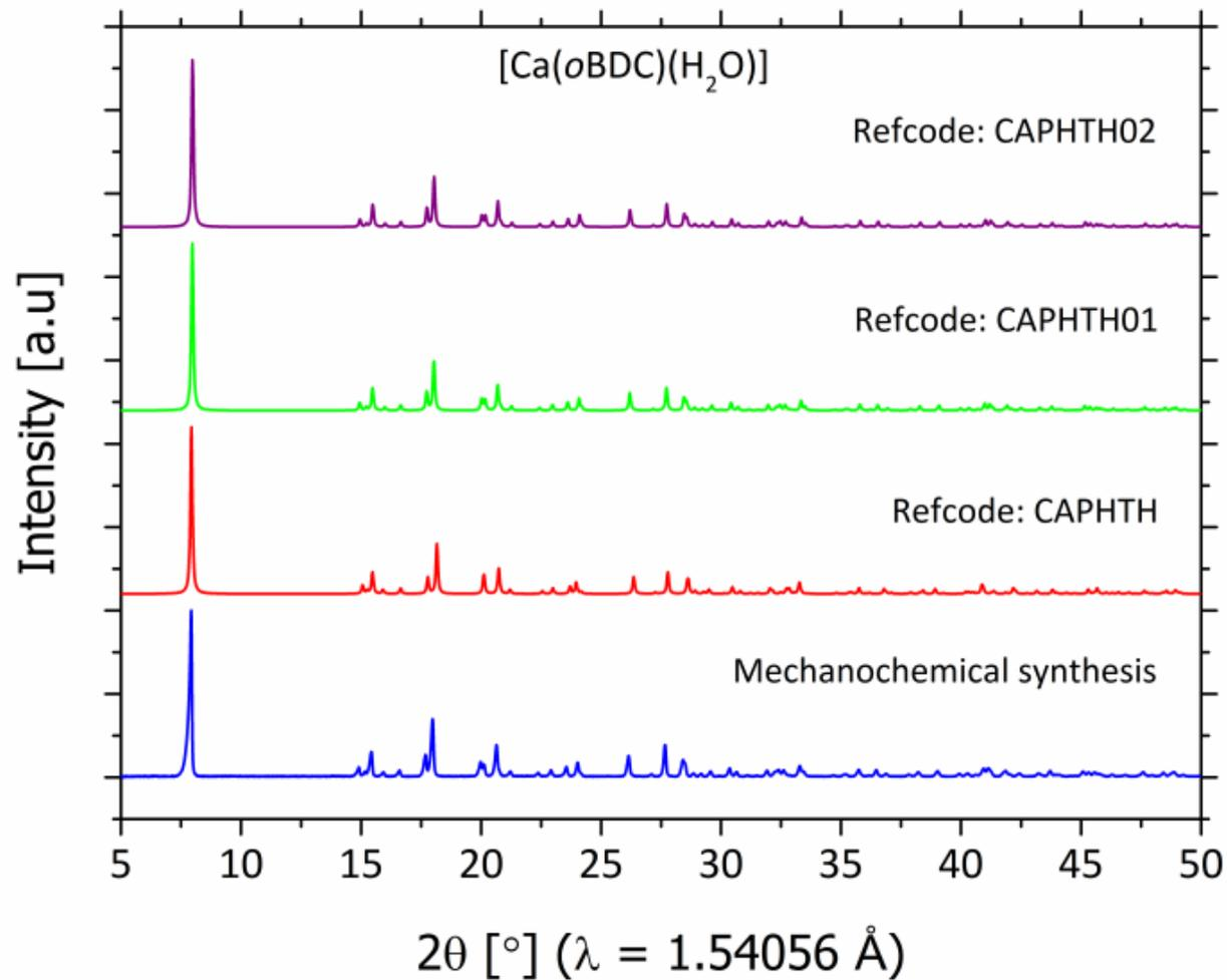
**Figure S1.** The PXRd patterns of  $[\text{Ca}(\text{oBDC})(\text{H}_2\text{O})]$  (1). The measured PXRd pattern of 1 obtained after milling (blue PXRd pattern) compared to the simulated PXRd data from the reported crystal structures by Gupta *et al.* (Refcode: CAPHTH, red PXRd pattern), Schuckmann *et al.* (Refcode: CAPHTH01, green PXRd pattern), and Zhang *et al.* (Refcode: CAPHTH02, purple PXRd pattern).
