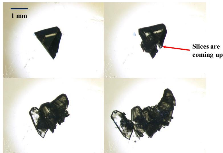
**Fig. S9** Stepwise shearing of THP-4Cl3NB crystal.
