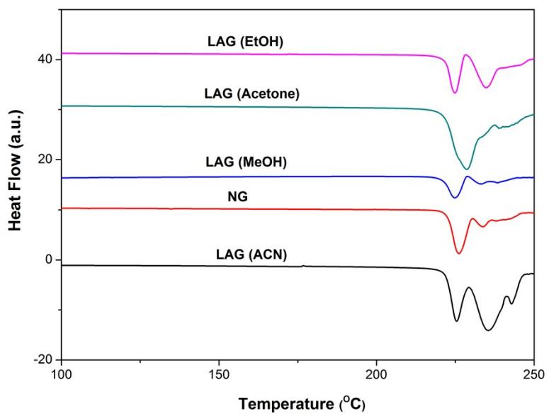
**Fig. S10** DSC thermogram of compositions obtained from different solvents (LAG) and neat grinded (NG) samples of THP-ACZ co-crystal.
