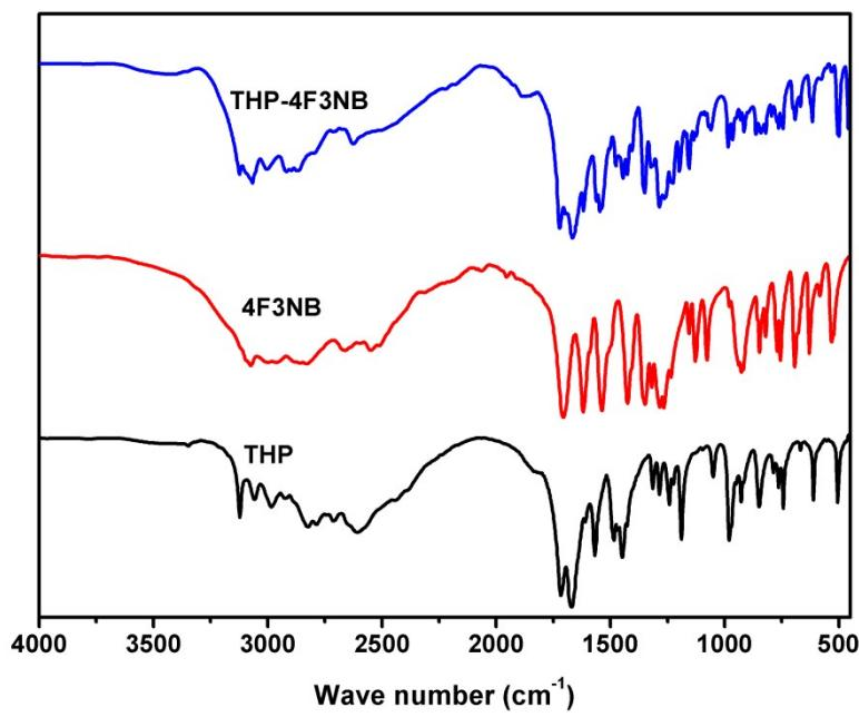
**Fig. S5** Comparison of FTIR spectra of THP, 4F3NB and its co-crystal, THP-4F3NB.
