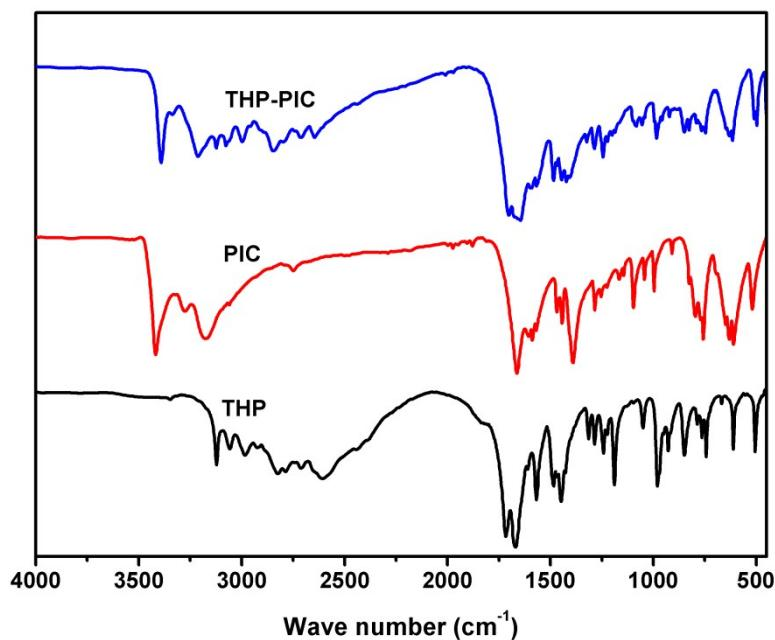
**Fig. S2** Comparison of FTIR spectra of THP, PIC and its co-crystal, THP-PIC.
