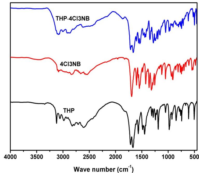
**Fig. S4** Comparison of FTIR spectra of THP, 4Cl3NB and its co-crystal, THP-4Cl3NB.
