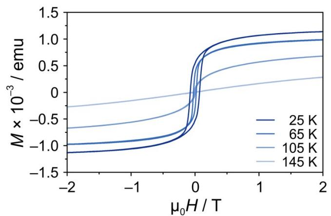
**Fig. S4** Hysteresis curves in the field range of  $\pm 2$  T obtained at different temperatures of 25 K, 65 K, 105 K and 145 K on a polymer-templated mesostructured PCMO thin film heated at 750 °C.
