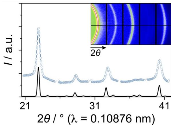
**Fig. S3** Synchrotron-based 1D and 2D GIWAXS patterns of a polymer-templated mesostructured PCMO thin film heated at 750 °C. For data analysis, DPDAK 1.2.0 was used and a geometric correction was performed on the data. The GIWAXS and SAED results are in agreement and demonstrate that the sol-gel derived material is single-phase after calcination and crystallizes in the orthorhombic space group *Pnma*.
