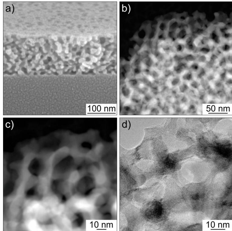
**Fig. S1** Electron microscopy of polymer-templated mesostructured PCMO thin films heated at 750 °C. (a) Cross-sectional SEM, (b, c) HAADF STEM and (d) HRTEM micrographs demonstrating both the structural integrity and crystallinity of the sol-gel derived material.
