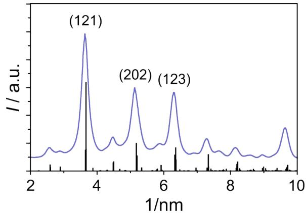
**Fig. S2** Radial integration pattern of SAED data (see Fig. 1e in the manuscript). The reflections match the ICSD reference code 56634 for  $\text{Pr}_{0.7}\text{Ca}_{0.3}\text{MnO}_3$  with an orthorhombic structure with space group *Pnma*.
