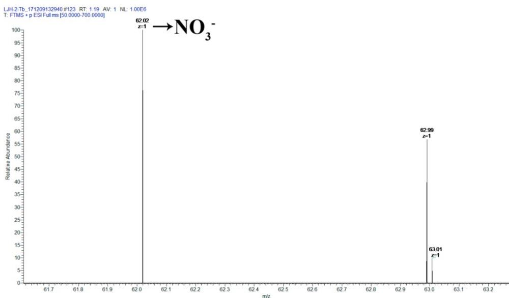
**Figure S6** Electrospray-ionization mass spectrometry (ESI-MS) of **1-Ln**
