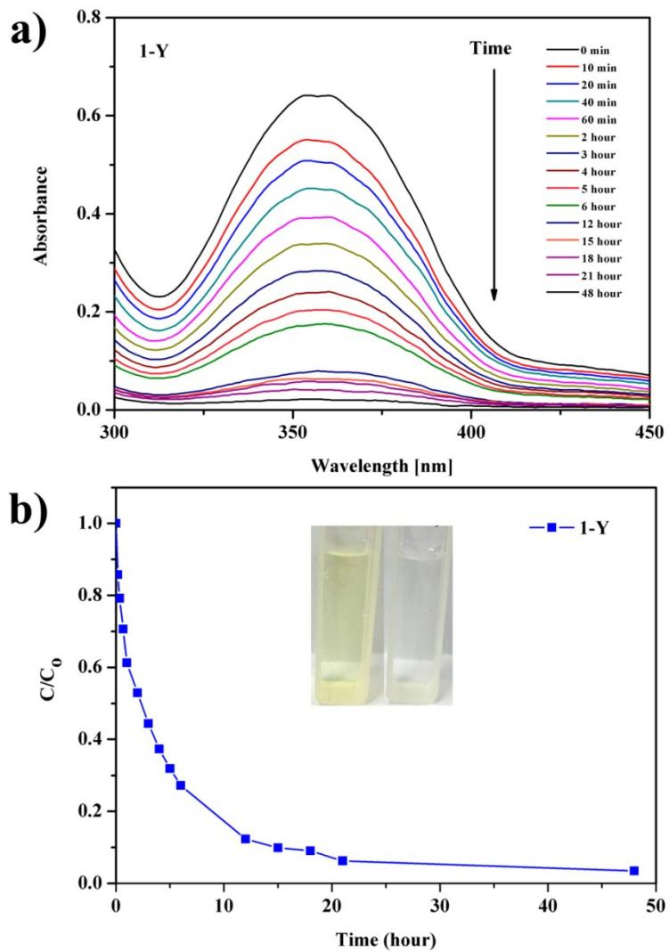
**Figure S11 (a)** UV/Vis spectra of  $\text{K}_2\text{Cr}_2\text{O}_7$  aqueous solution during anion exchange with **1-Y**. (b) The adsorption rate of **1-Y**. Inset: The photographs show the color of the  $\text{K}_2\text{Cr}_2\text{O}_7$  solution before (left) and after (right) ion-exchange for 48 h.
