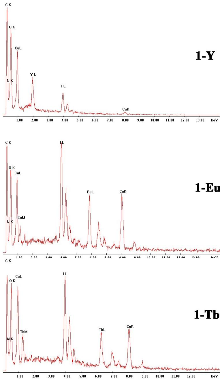
**Figure S1** Energy-dispersive X-ray spectroscopy of **1-Ln**.
