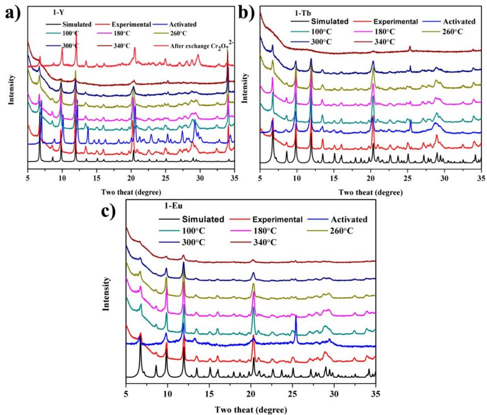
**Figure S7** The simulated and temperature dependent PXRD patterns of **1-Ln** from room temperature to 340 °C.
