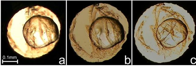
**Fig. S2.** The crystal sample of HCE in the high-pressure diamond-anvil cell at: 3.19 (a), 4.02 (b) and 5.42 GPa (c). Two small ruby chips, used as pressure markers, are visible in the upper part of the high pressure chamber. The cellulose fibres were used to fix the crystal sample in the cell.
