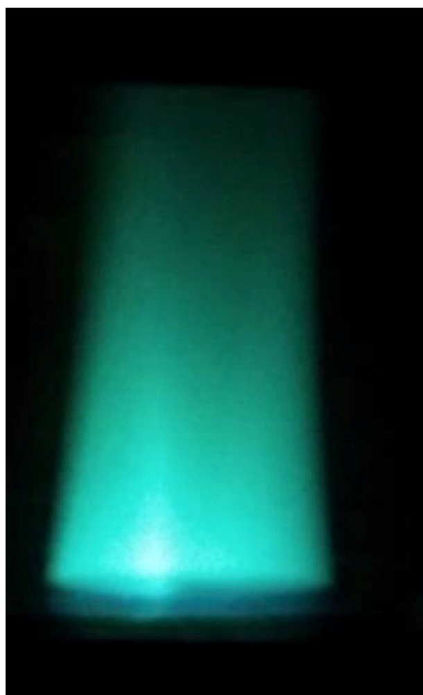
Fig. S4 The luminescence photograph of CDs under the excitation of 440 nm.
