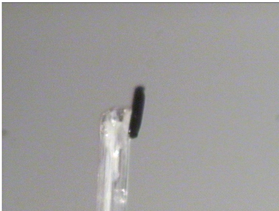
Figure S13 Crystal of 4 . The raw data were unfortunately lost due to a malfunction of a hard drive; however it is reasonable to assume that the longest axis of the crystal corresponds to the direction [100] , which is the direction of stacking.
