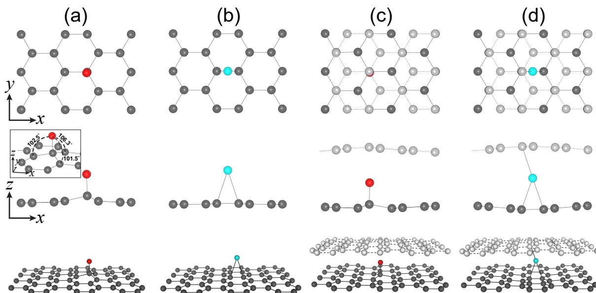
FIG. S2: Orthogonal top, side views and perspective side views of the O/graphene and F/graphene transition states. In the inset of (a), three different C–C–O angles are given.
