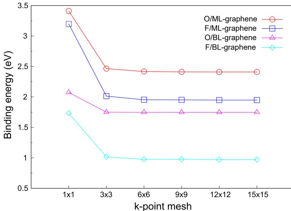
FIG. S1: Binding energies of O/graphene and F/graphene systems with different k-point meshes
