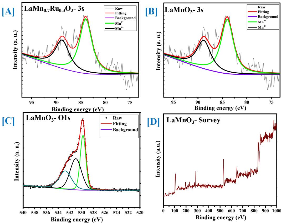
**Fig. S1** XPS spectra of LaMn<sub>0.7</sub>Ru<sub>0.3</sub>O<sub>3</sub> [A] Mn 3s, [B] LaMnO<sub>3</sub> Mn 3s, [C] LaMnO<sub>3</sub> O 1s core levels and [D] LaMnO<sub>3</sub> survey spectrum.
