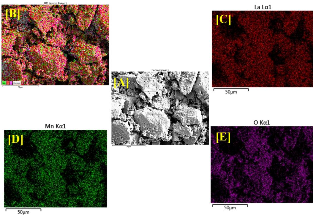
**Fig. S4** [A] FESEM image of LaMnO<sub>3</sub>, [B] EDX mapping of [A], elemental distribution of [C] La, [D] Mn, [E] O in [B].
