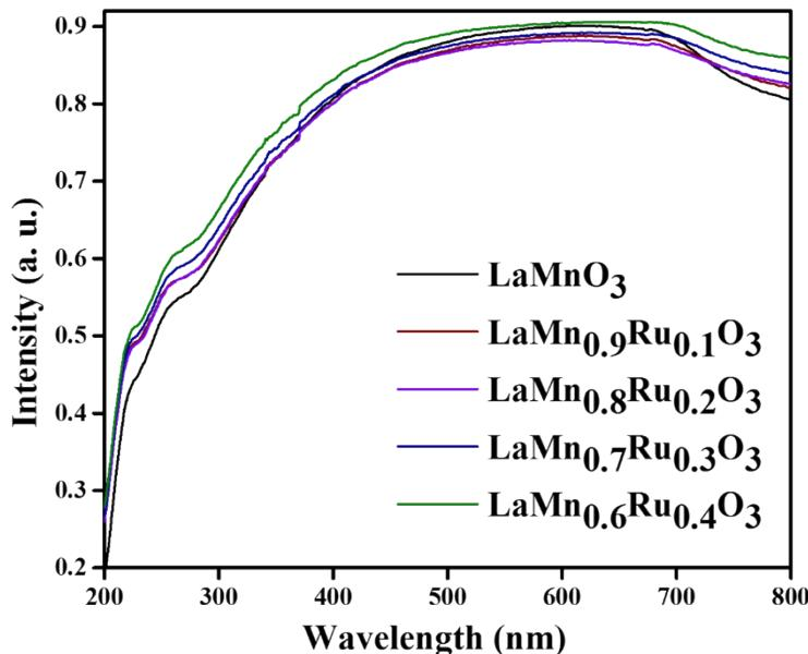
**Fig. S2** UV-Visible diffuse reflectance spectra of LaMn<sub>1-x</sub>Ru<sub>x</sub>O<sub>3</sub> (x = 0.0-0.4).
