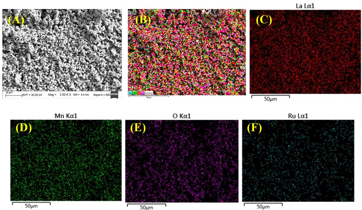
**Fig. S3** [A] FESEM image of  $\text{LaMn}_{0.7}\text{Ru}_{0.3}\text{O}_3$ , [B] EDX mapping of [A], elemental distribution of [C] La, [D] Mn, [E] O and [F] Ru in [B].
