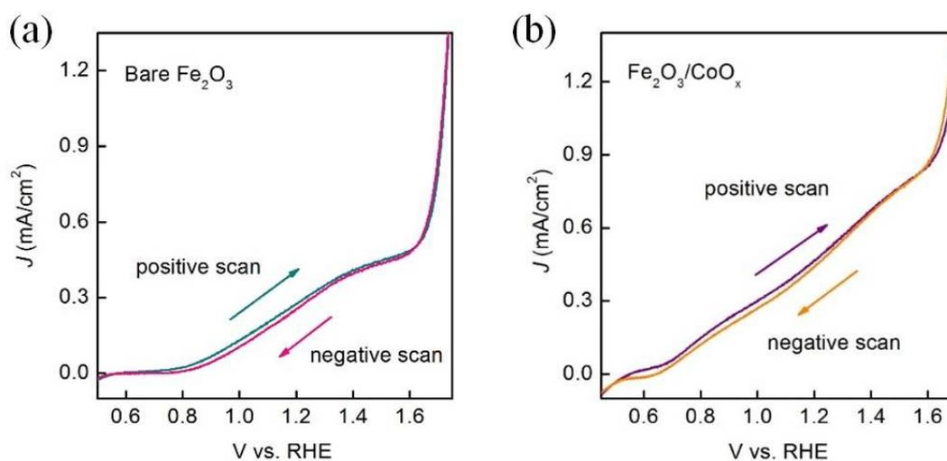
**Fig. S8.**  $J$ - $V$  curves with opposite scan directions on (a) bare (left) and (b)  $\text{CoO}_x$  coated hematite (right) photoanode. Positive scan means the applied potential start from low value, while the negative scan starts from high potential value.
