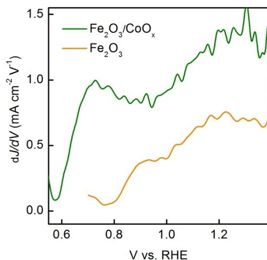
**Fig. S3.** First-order derivative of the photocurrent density as a function of voltage was calculated. The onset potential is defined as the voltage at which  $dJ/dV \geq 0.2 \text{ mA cm}^{-2} \text{ V}^{-1}$ . The onset potential was read as  $0.85 \text{ V}_{\text{RHE}}$  and  $0.60 \text{ V}_{\text{RHE}}$  for  $\text{Fe}_2\text{O}_3$  and  $\text{Fe}_2\text{O}_3/\text{CoO}_x$ , respectively.
