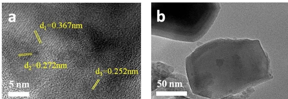
**Fig. S2.** (a) High-resolution TEM image of hematite with ALD  $\text{CoO}_x$  modification layer. (b) TEM image of single hematite nano-structure unit.
