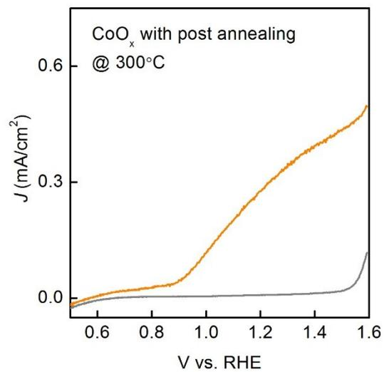
**Fig. S11.** *J-V* curves for CoO<sub>x</sub> coated hematite photoanode with post annealing in air at 300 °C. Compared to as-prepared CoO<sub>x</sub>/Fe<sub>2</sub>O<sub>3</sub> photoanode, turn on potential shifts positively to 0.9 V<sub>RHE</sub> after thermal treatment.
