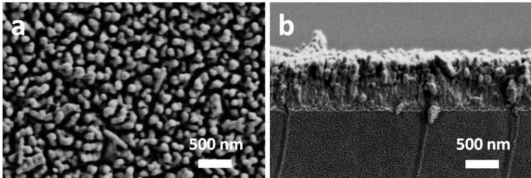
**Fig. S1.** Top-view (a) and side-view (b) SEM images of bare hematite nanostructured film. The scale bar is 500 nm.
