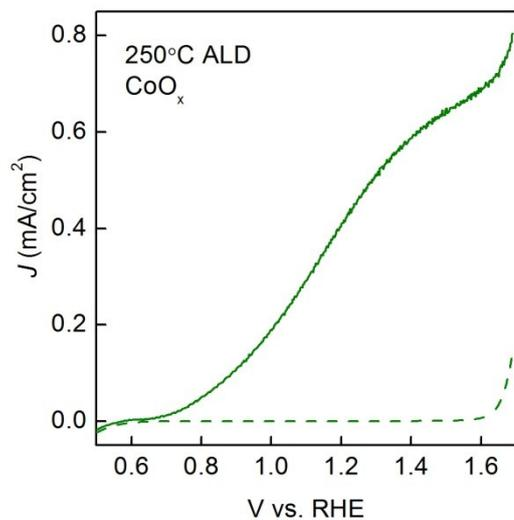
**Fig. S5.** Polarization  $J$ - $V$  curve for CoO<sub>x</sub> coated hematite photoanode with growth temperature at 250 °C. Water oxidation turn on potential is around 0.7 V<sub>RHE</sub>.
