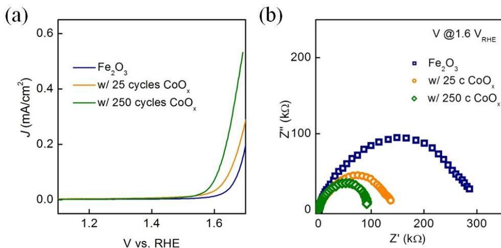
**Fig. S9.** (a) Dark  $J$ - $V$  curves on hematite with 0 , 25 and 250 cycles of ALD CoO<sub>x</sub> overlayer. Hematite with 250 cycles of ALD CoO<sub>x</sub> with the highest OER activity exhibits the earliest Von potential. (b) Representative Nyquist plot data for various hematite photoanodes collected in dark condition.
