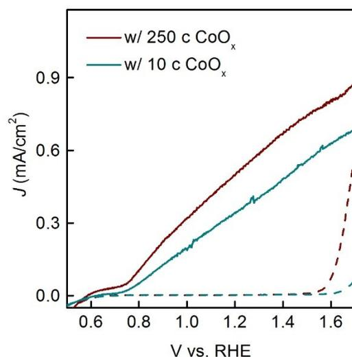
**Fig. S4.** Steady-state  $J$ - $V$  curves for hematite photanode with 10 cycles and 250 cycles of ALD  $\text{CoO}_x$  overlayer. Solid and dashed curves represent the response collected in light and dark condition respectively. Both light curves express improvement in turn on potential compared to bare hematite film.
