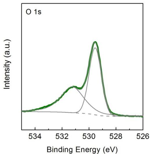
**Fig. S6.** XPS characterizations of O 1s on CoO<sub>x</sub> coated hematite sample. Green curve is the raw data and grey lines are fitted results.
