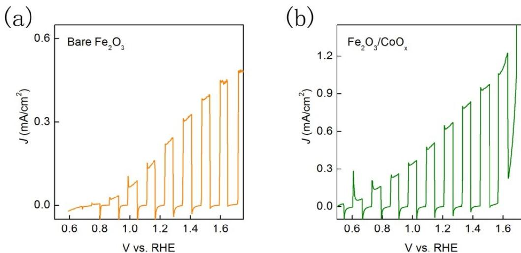
**Fig. S7.** Polarization  $J$ - $V$  curves of bare  $\text{Fe}_2\text{O}_3$  (a) and  $\text{Fe}_2\text{O}_3/\text{CoO}_x$  (b) tested in 1 M KOH, under chopped AM 1.5 illumination. Positive and negative spikes show up when light was switched on and off.
