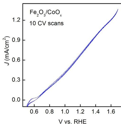
**Fig. S10.** CV scans on CoO<sub>x</sub> coated hematite photoanode. CV scan was done for 10 times with a scan rate of 10 mV/s. Negligible oxidation or reduction features are exhibited in the CV results.
