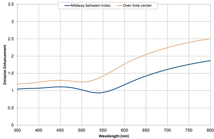
**Figure S2.** Enhanced emission from a small dipole placed 20 nm above the Au-Nanohole surface.
