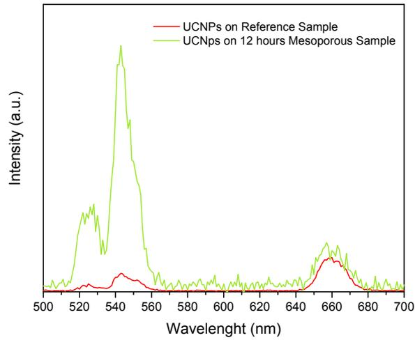
**Figure S7.** UCPL intensity of  $\beta$ -NaYF<sub>4</sub>:Yb<sup>3+</sup>, Er<sup>3+</sup> nanoparticles on reference sample and on Au mesoporous sample with a 12-hour dealloying time, directly without any SiO<sub>2</sub> spacer layer. This measurement shows about 15 times quenching effect at 541 nm emission and about 1.5 times quenching effect at 656 nm emission.
