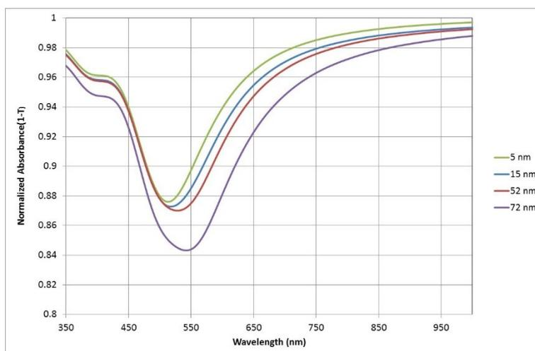
**Figure S1.** Absorption (1-Transmission) for 5 nm, 15 nm, 52 nm and 72 nm nanoholes in a 100 nm Au film.
