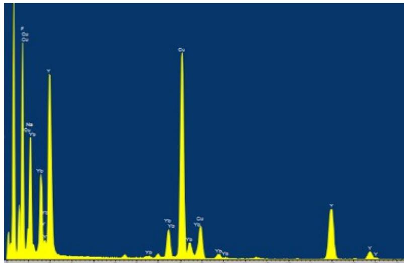
**Figure S5.** TEM energy dispersive X-Ray (EDX) spectrum of the UCNPs, collected from the same area as Figure 3a. The figure confirms the existence of elemental Na, Y, Yb, and F in UCNPs. The absence of Er detections was due to the very small amount of Er present in UCNPs, which was out of the limit of the instrumental sensitivity. The Cu signal element was from the copper TEM grid.
