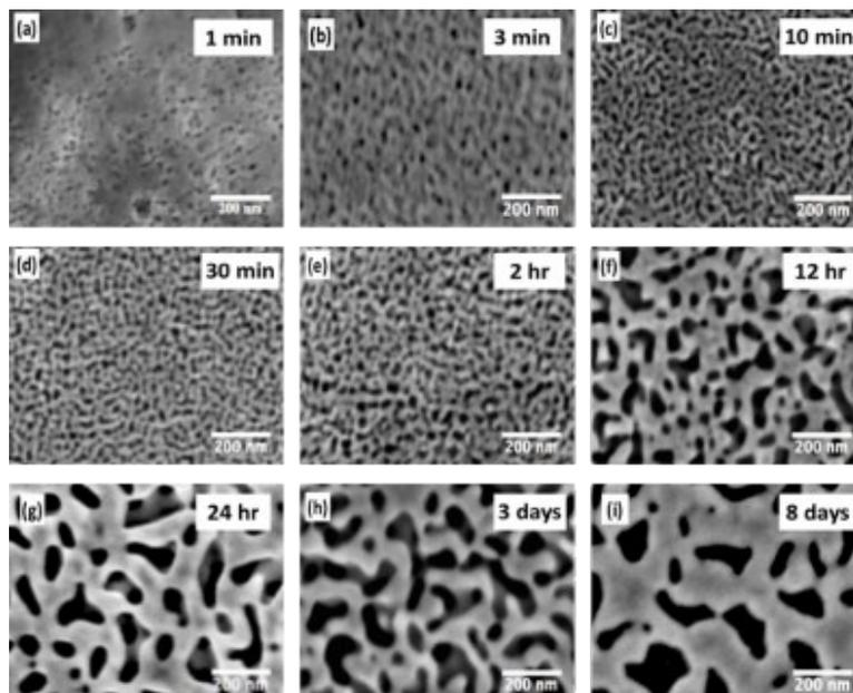
**Figure S6.** (a-i) Top-view SEM micrographs showing the porosity evolution of Au mesoporous films with respect to different dealloying time, ranging from 1minute to 8 days.
