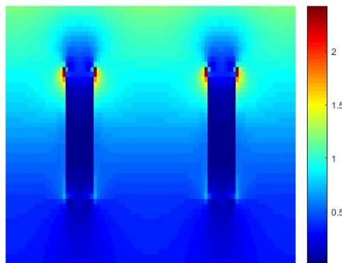
**Figure S3.** Electric field enhancement at 980 nm (in the cross section through the centre of the holes). The incident plane wave was polarised parallel to the Au surface.
