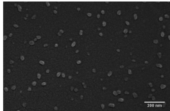
**Figure S9.** Top-view SEM micrographs showing the reference sample - glass substrate with UCNPs on the top. (With 120K magnification).
