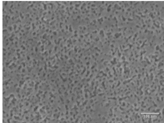
**Figure S8.** Top-view SEM micrographs showing the Au mesoporous film with 3 minutes dealloying time. (With 100K magnification).
