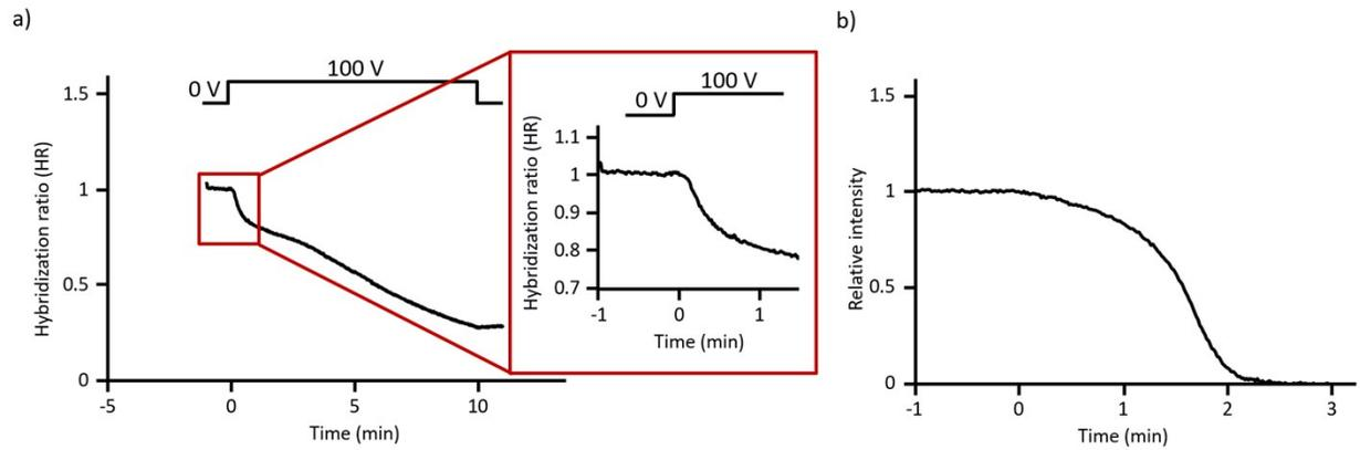
Figure S7. a) Hybridization ratio over time of U15-GNP5 under 100V (Fig. 1c from main text) and inset of the slow kinetics. b) Relative intensity of electrophoresing U15-GNP5 in a hydrogel without anchor under 100V in a vertical chamber.
