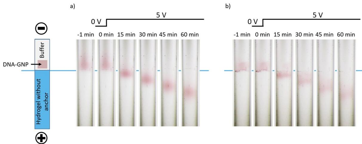
Figure S8. Band over time of DNA-GNP in a hydrogel without anchor under 5V in a vertical chamber. a) U15-GNP5. (b) U15-GNP10.
