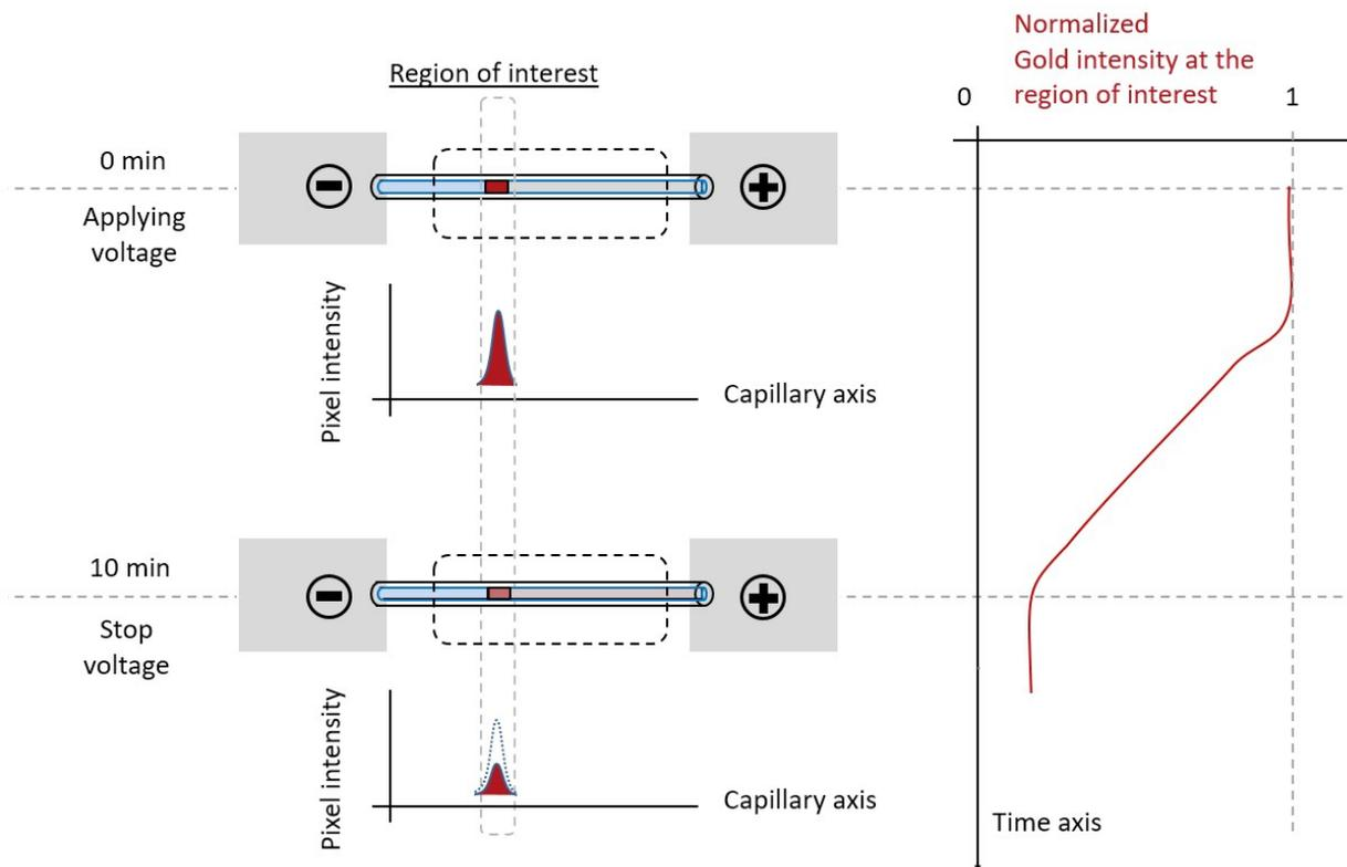
Figure S5. Method for obtaining hybridization ratio. The reddish color intensity distribution inside the capillary is shown at time zero and after 10 min (left), and its representation over time is shown (right)
