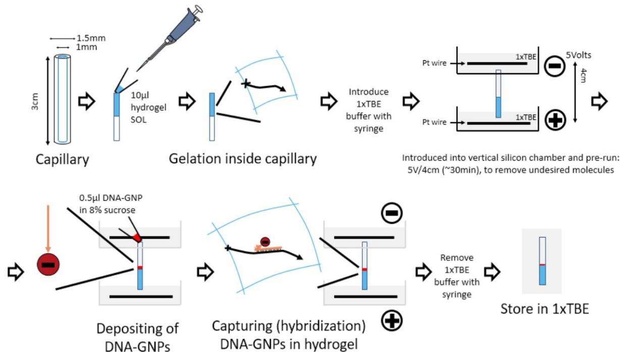
Figure S3. Scheme of the preparation of capillary
