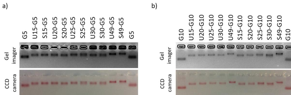
Figure S2. 2% gel electrophoresis assay for both 5nm and 10nm GNP. Gel imager uses white EPI light source and 530/28 filter. a) 5 nm GNP. b) 10 nm GNP.
