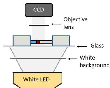
Figure S4. CCD recording setup for the dehybridization time evolution.
