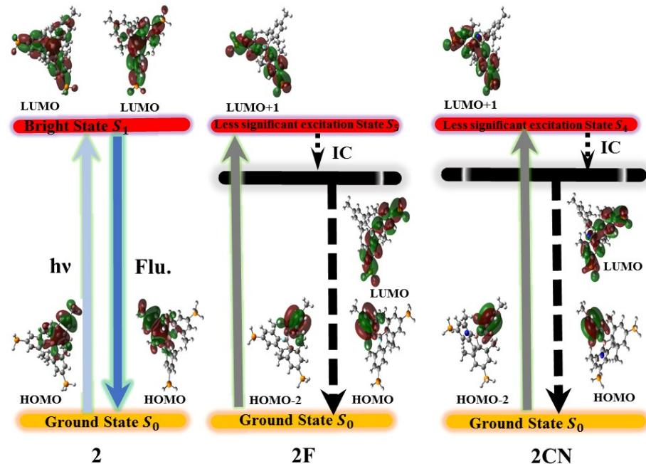
Figure S8: Scheme of the different mechanisms of fluorescence emission for **2**, **2F** and **2CN**.
