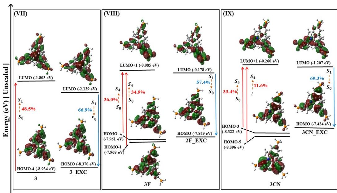
Figure S5: Calculated FMO energies for (VII) **3** in ground state and excited state (**3\_EXC**) (VIII) **3F** in ground state and excited state (**3F\_EXC**) and (IX) **3CN** in ground state and excited state (**3CN\_EXC**) at CAM-B3LYP/6-31G(d) level using CPCM solvation model.
