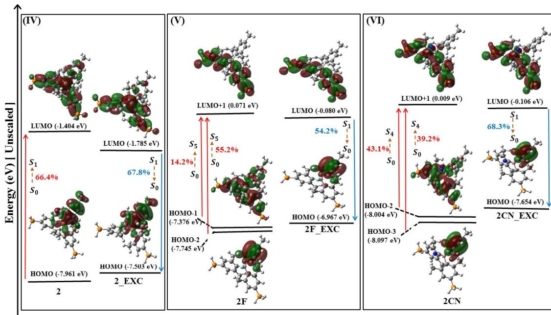
Figure S4: Calculated FMO energies for (IV) **2** in ground state and excited state (**2\_EXC**) (V) **2F** in ground state and excited state (**2F\_EXC**) and (VI) **2CN** in ground state and excited state (**2CN\_EXC**) at CAM-B3LYP/6-31G(d) level using CPCM solvation model.
