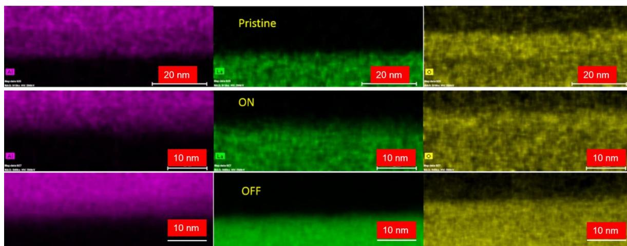
**Figure S1.** EDS maps of individual elements in pristine/ON/OFF state samples, showing no diffusion of La (Ni) into the interlayer.
