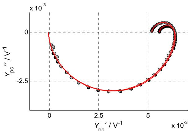
Figure S2: IMPS measurements at 1.35 VRHE with the white LED (4300 K) for 50 mW/cm<sup>2</sup> (grey symbols) and 100 mW/cm<sup>2</sup> (black symbols) bias light intensities. Obtained fits are also shown (red lines).
