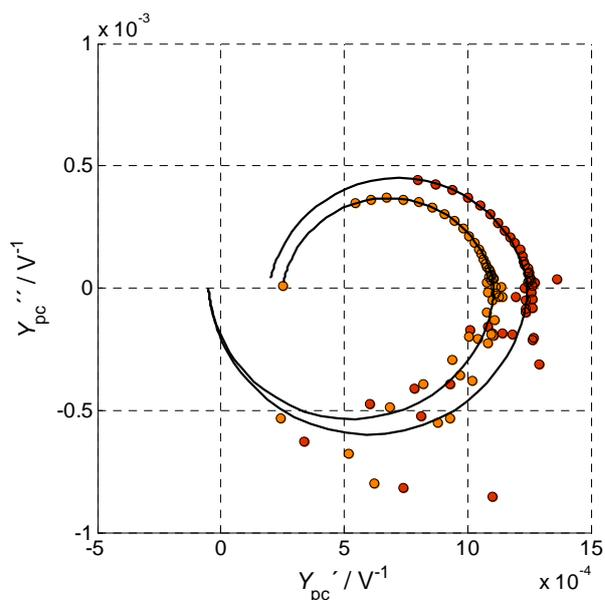
Figure S4: IMPS measurements at 1.35 VRHE with the orange LED (590 nm) for 4.5 mW/cm<sup>2</sup> (orange symbols) and 9 mW/cm<sup>2</sup> (red symbols) bias light intensities. Obtained fits are also shown (black lines).
