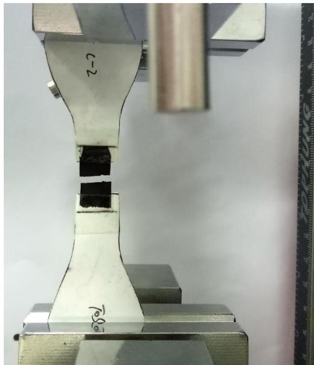
Figure S4 Broken sample of PPy film with a polymerization charge of 2 C·cm<sup>-2</sup>
