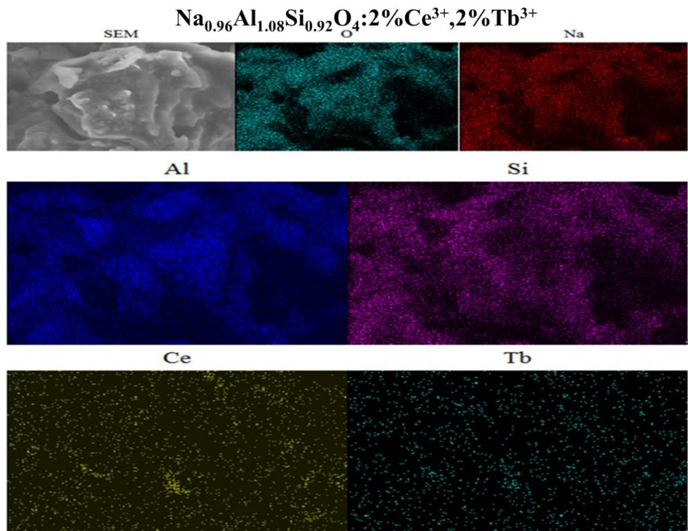
Fig.S6 The analysis of SEM and mapping for each element in NAS:2%Ce<sup>3+</sup>,2%Tb<sup>3+</sup>.
