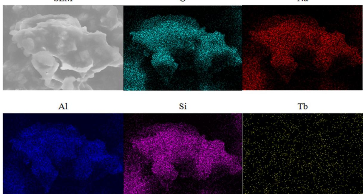
Fig.S4 The analysis of SEM and mapping for each element in NAS:2%Tb<sup>3+</sup>.
