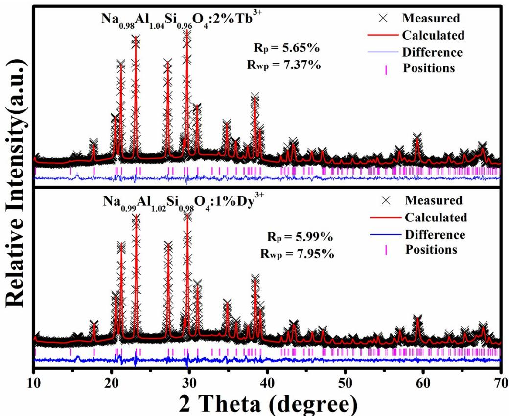
Fig.S1 Rietveld refinement of the powder XRD pattern of NAS:2%Tb<sup>3+</sup> and NAS:1%Dy<sup>3+</sup>.
