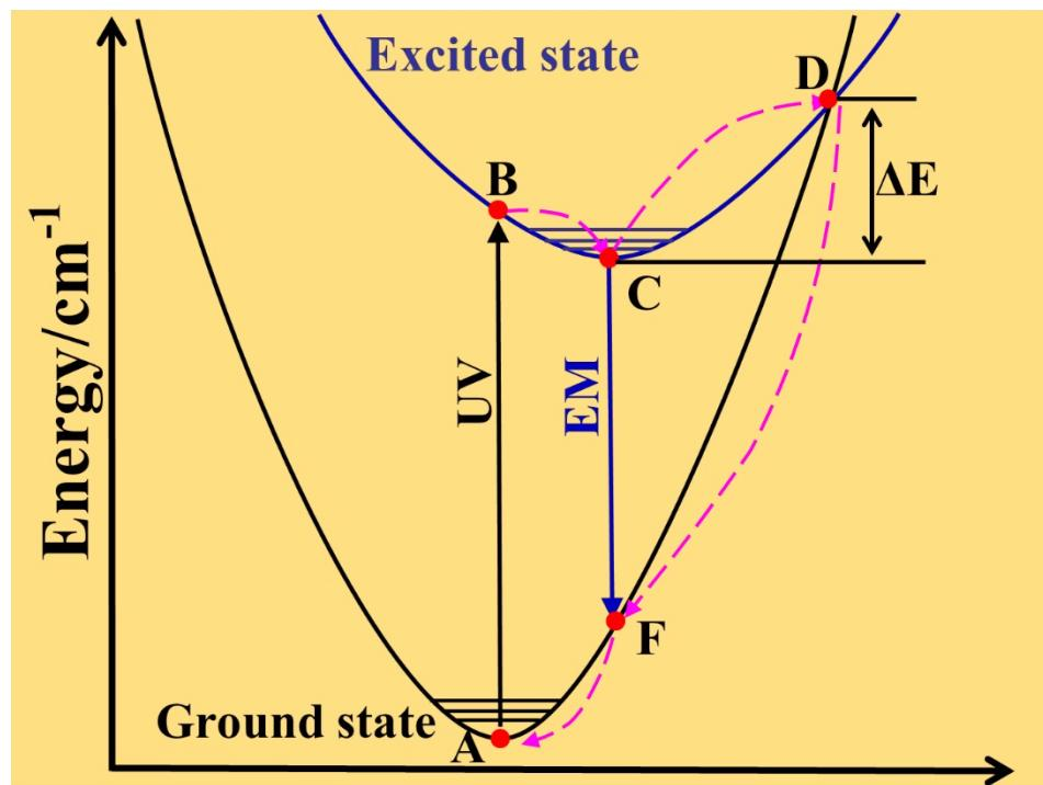
Fig.S11 The schematic of configurational coordinate diagram for general mechanism of temperature-dependent emission of phosphor.
