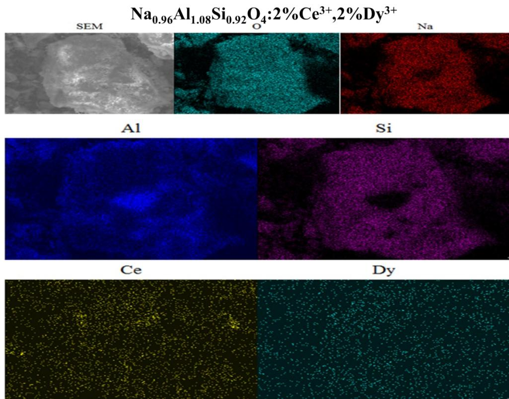
Fig.S7 The analysis of SEM and mapping for each element in NAS:2%Ce<sup>3+</sup>,2%Dy<sup>3+</sup>.
