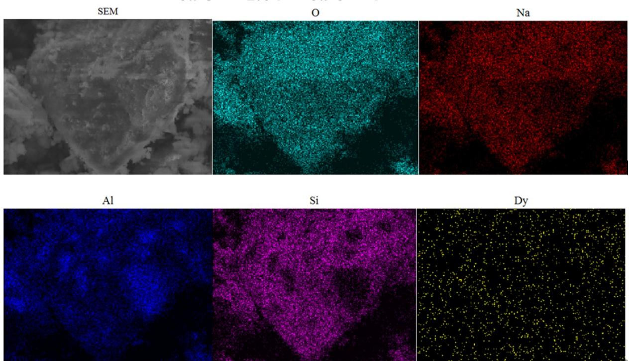
Fig.S5 The analysis of SEM and mapping for each element in NAS:2%Dy<sup>3+</sup>.
