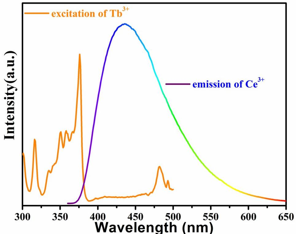
Fig.S9 Spectral overlap between the photoluminescence excitation spectrum of NAS:Tb<sup>3+</sup> (orange line) and the photoluminescence spectrum of NAS:Ce<sup>3+</sup> (colorized line).
