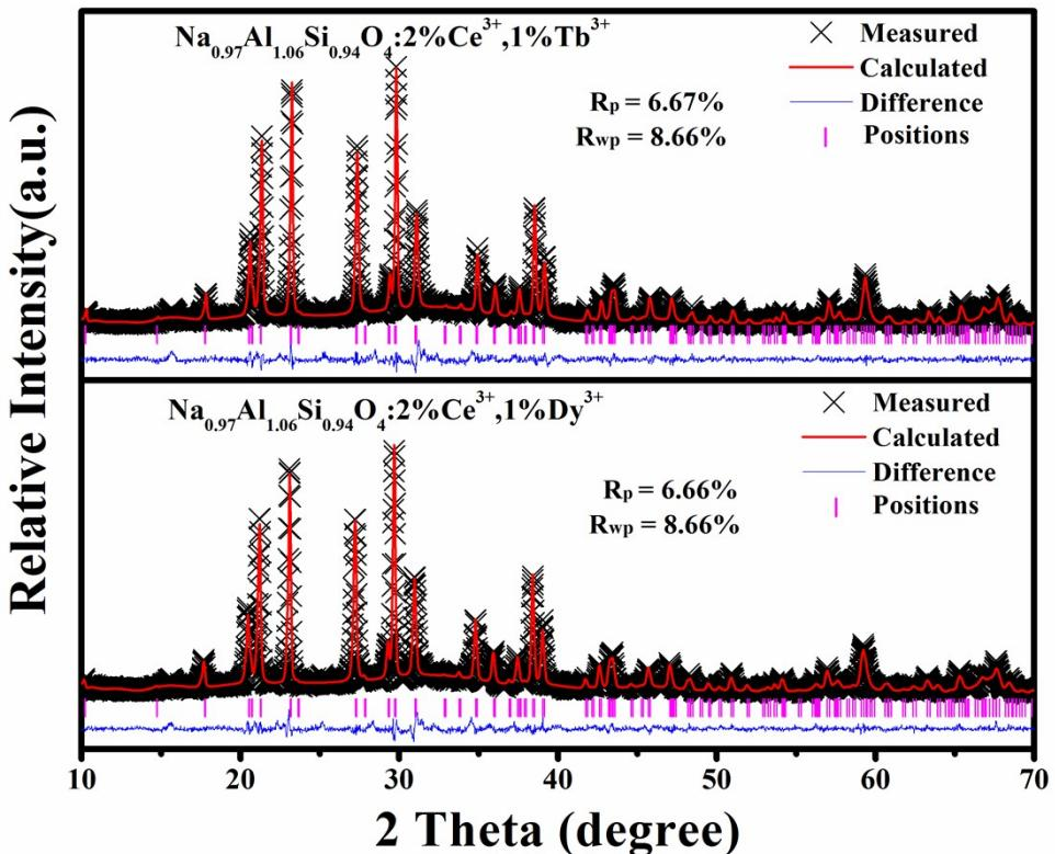
Fig.S2 Rietveld refinement of the powder XRD pattern of  $\text{NAS}:2\%\text{Ce}^{3+},1\%\text{Tb}^{3+}$  and  $\text{NAS}:2\%\text{Ce}^{3+},1\%\text{Dy}^{3+}$ .
