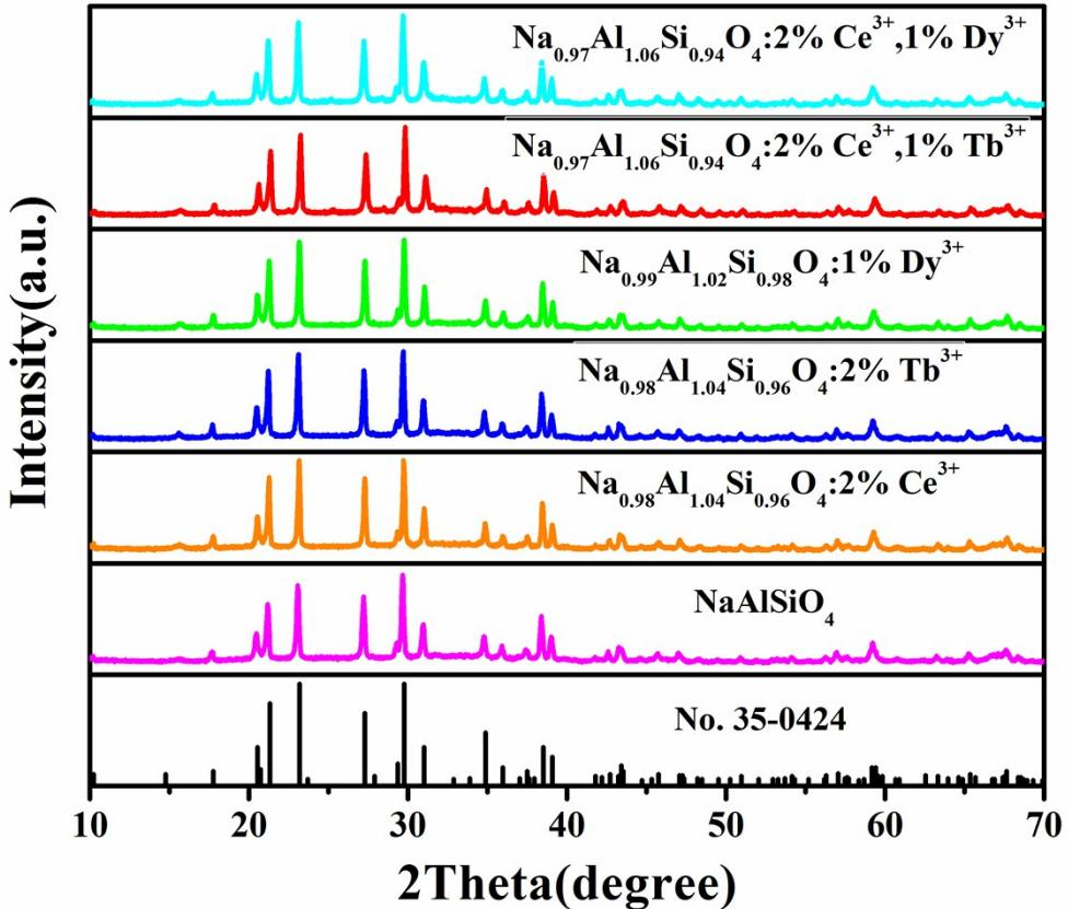
Fig.S3 The representative XRD patterns for  $\text{Ce}^{3+}/\text{Tb}^{3+}/\text{Dy}^{3+}$  doped NAS samples.
