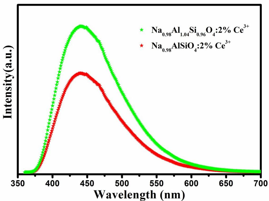
Fig. S8 The comparison of luminous intensity of NAS:2%Ce<sup>3+</sup> before and after the charge compensation.
