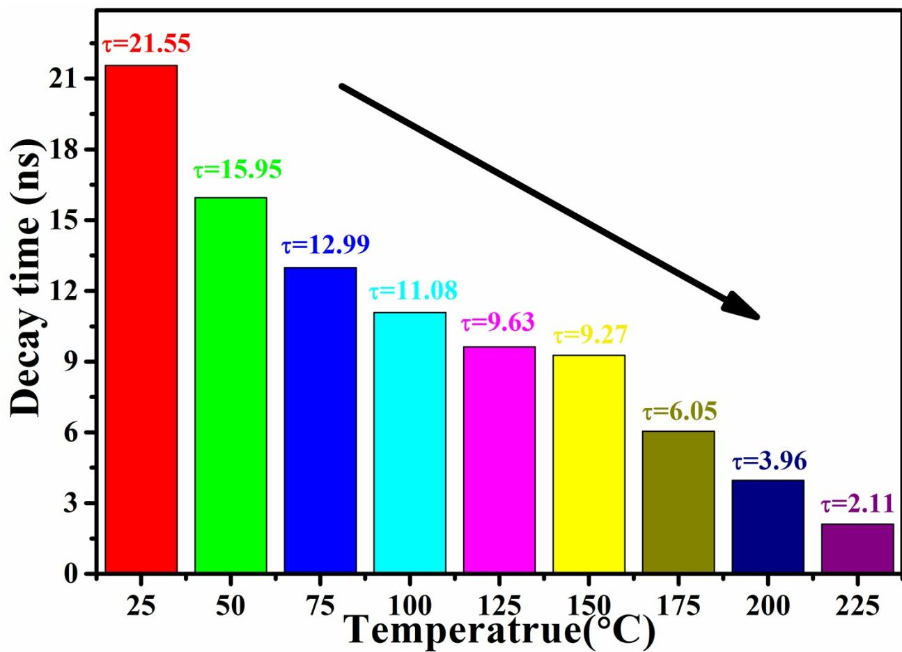
Fig.S12 The dependence of the average lifetimes ( $\tau$ ) on temperature for NAS:2%Ce<sup>3+</sup>.
