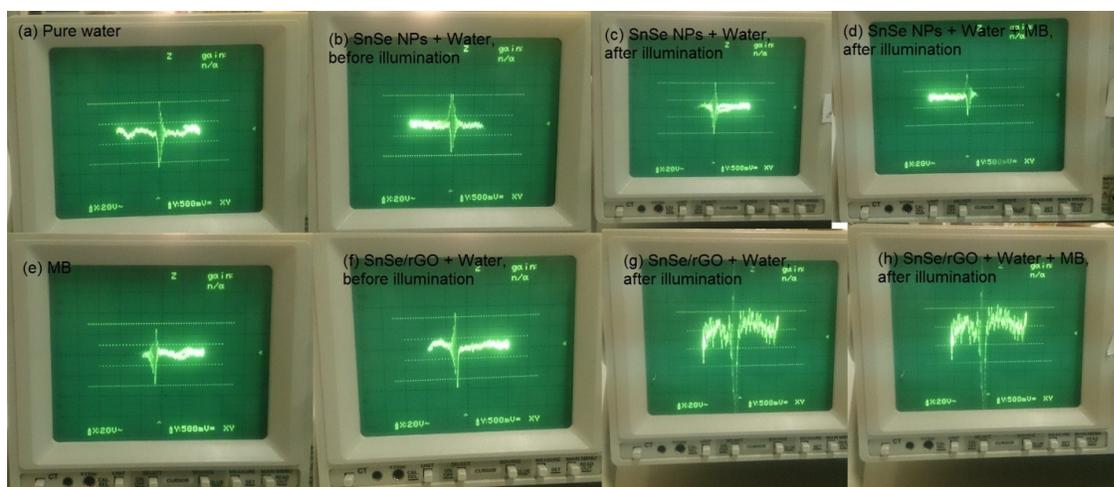
**Fig. S3** ESR peak of (a) pure water, (b) SnS NSs + water before illumination, (c) SnS NSs + water after illumination, (d) SnSe NSs + water + MB after illumination, (e) MB solution, (f) SnSe/rGO + water before illumination, (g) SnSe/rGO + water after illumination, (h) SnSe/rGO + water + MB after illumination.
