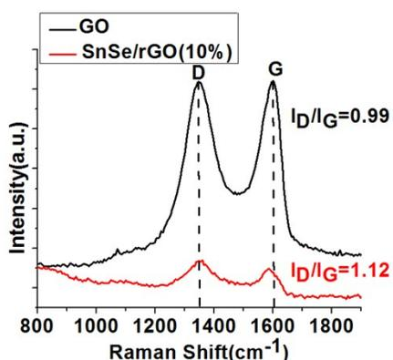
**Fig. S1** Raman spectrum of the GO sheets and SnSe/rGO nanocomposites.
