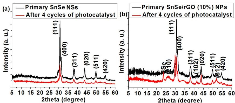
**Fig. S5** XRD patterns of primary and after four cycles photocatalytic activity of (a) the pristine SnSe NSs and (b) SnSe/rGO nanocomposites to remove MB.
