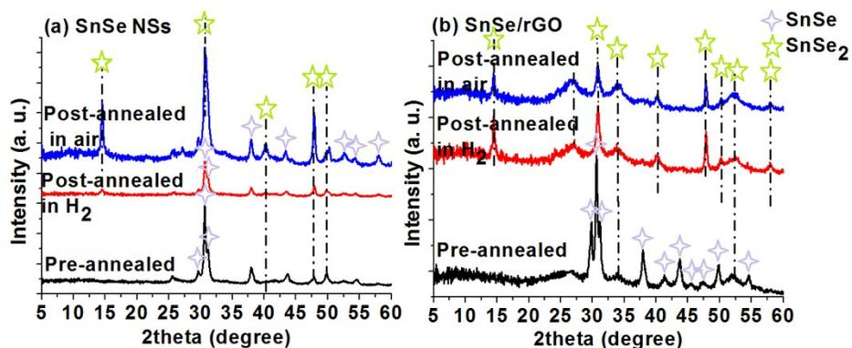
**Fig. S2** XRD patterns of the pre- and post-annealed of (a) the pristine SnSe NSs and (b) SnSe/rGO nanocomposites in hydrogen and air atmosphere.
