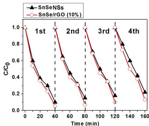
**Fig. S4** Reusability test of the pristine SnSe NSs and SnSe/rGO nanocomposites catalyst for the photodegradation of MB.
