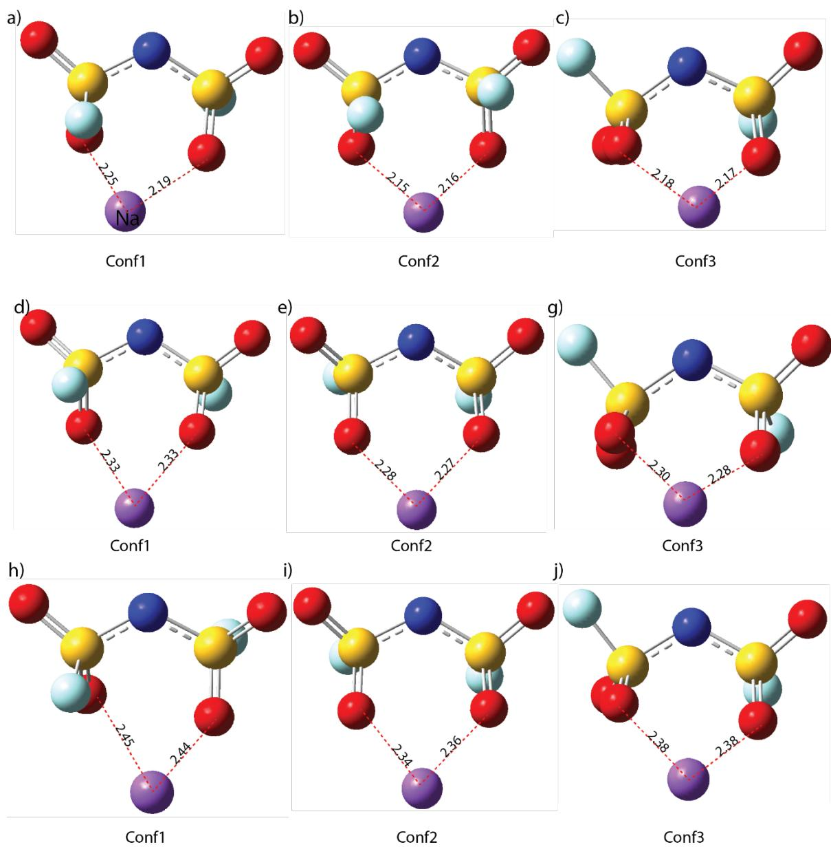
**Figure S2.** Optimized structures of LiFSI in a-c) gas phase, d-f)  $\text{CHCl}_3$  and h-j) DMSO.
