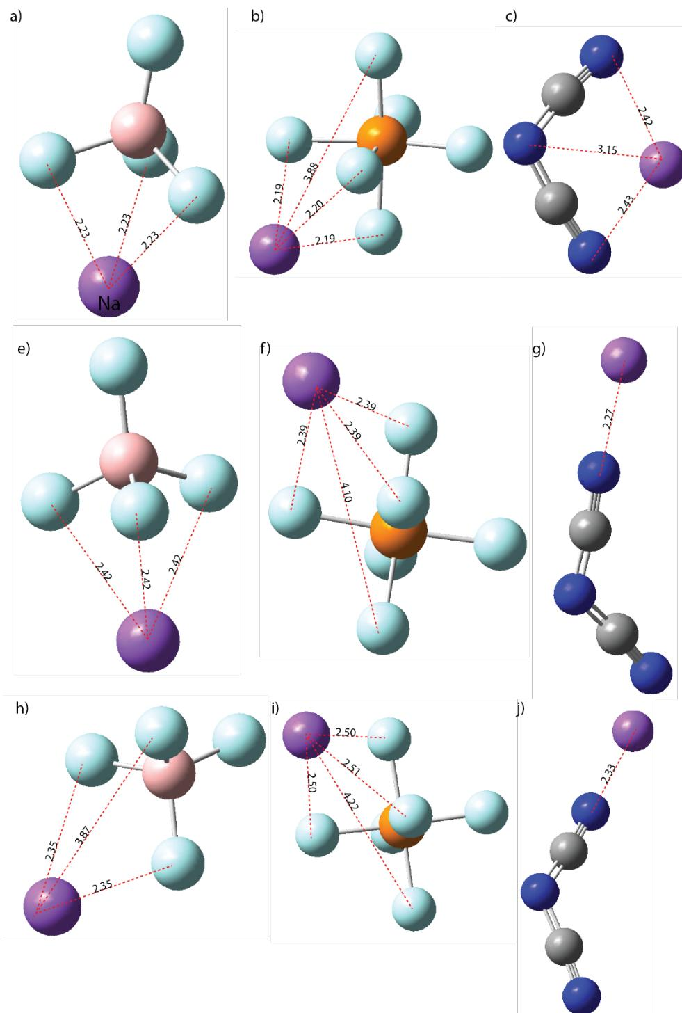
**Figure S4.** Optimized structures in gas phase a)  $\text{NaBF}_4$ , b)  $\text{NaPF}_6$ , c)  $\text{NaDCA}$ , in  $\text{CHCl}_3$  e)  $\text{NaBF}_4$ , f)  $\text{NaPF}_6$ , g)  $\text{NaDCA}$ , , in DMSO h)  $\text{NaBF}_4$ , j)  $\text{NaPF}_6$ , k)  $\text{NaDCA}$ ,
