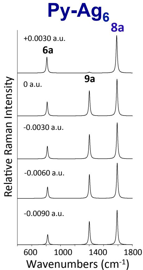
**Figure S3.** Effect of the electric field on the  $I_{k,CT}^{\text{preRR}(1)}$  intensities of Py-Ag<sub>6</sub> calculated by using the dimensionless displacements  $\Delta_{k,CTA1}$  reported in Table S3 of ref. 1 for the 6a, 9a and 8a modes. Electric fields labelled according to ref. 1. The value of  $\Delta_{9a,CTA1}=0.1606$  for +0.0030 a.u. seems to be wrong.
