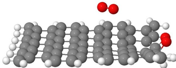
**Figure S4.** Optimized adsorption geometries for side-on adsorption of O<sub>2</sub> at the zigzag edge and basal plane of graphene.
