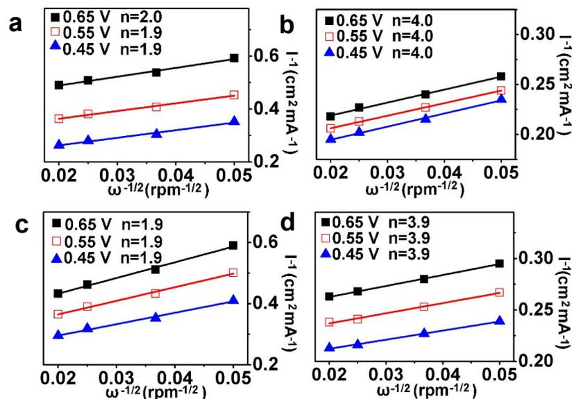
**Figure S3.** Koutecky–Levich plots of  $I^{-1}$  vs.  $\omega^{-1/2}$  of (a) graphene, (b) F-graphene, (c) MWCNTs, and (d) S-MWCNT electrodes in a 0.1 M KOH solution saturated with oxygen at different potentials.
