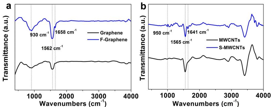
**Figure S2.** FTIR of (a) graphene and F-graphene and (b) MWCNTs and S-MWCNTs.
