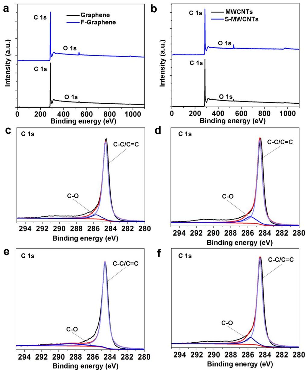
**Figure S1.** XPS spectra of (a) graphene and F-graphene and (b) MWCNTs and S-MWCNTs, C 1s of (c) graphene, (d) F-graphene, (e) MWCNTs and (f) S-MWCNTs.
