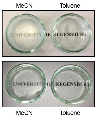
**Fig. S2** Proof of transparency of gels made in toluene (17 mg/mL) in comparison to gels made in MeCN (9 mg/mL). *Top:* Intact gels. *Bottom:* Gels destroyed using a spatula.
