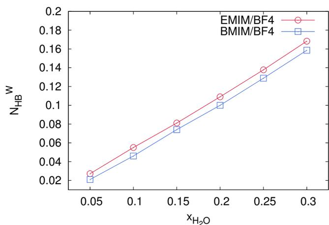
**Fig. 1** Number of hydrogen bonds  $N_{\text{HB}}^{\text{W}}$  between water molecules at different mole fractions of water in EMIM/BF4 (red circles) and BMIM/BF4 (blue squares). The lines are guides for the eyes only.
