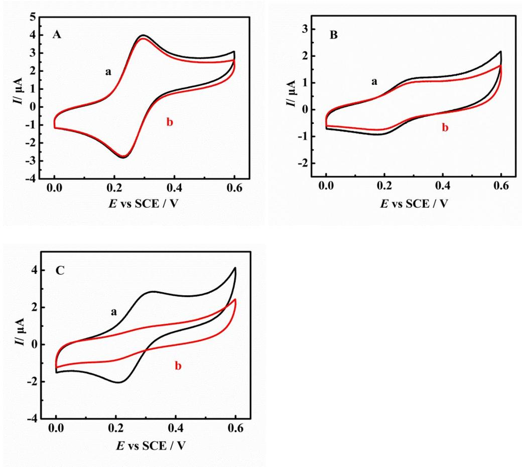
**Fig. S4** CVs of 0.5 mM FCA at 0.1 V s<sup>-1</sup> in pH 9.0 buffers at 37 °C at (A) bare Au, (B) PNIPAM and (C) PAPBA film electrodes with (a) 0 and (b) 0.2 M glucose, respectively.
