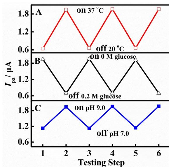
**Fig. S6** Dependence of CV  $I_{pa}$  of 0.5 mM FCA at 0.3 V for P(NIPAM-*co*-APBA) films at 0.01 V s<sup>-1</sup> in buffers containing 5 mM NADH on (A) the solution temperature switched between 20 and 37 °C at pH 9.0, (B) the glucose concentration cycled between 0 and 0.2 M at pH 9.0 and 37 °C, and (C) the solution pH switched between 7.0 and 9.0 at 37 °C.
