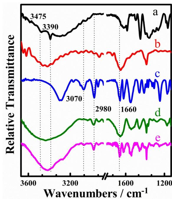
**Fig. S2** IR spectra of (a) APBA, (b) PAPBA, (c) NIPAM, (d) PNIPAM and (e) P(NIPAM-*co*-APBA) samples.
