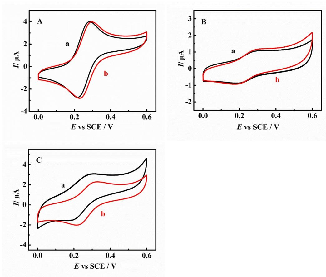
**Fig. S5** CVs of 0.5 mM FCA at  $0.1 \text{ V s}^{-1}$  and at  $37 \text{ }^\circ\text{C}$  at (A) bare Au, (B) PNIPAM and (C) PAPBA film electrodes in (a) pH 7.0 and (b) pH 9.0 buffers, respectively.
