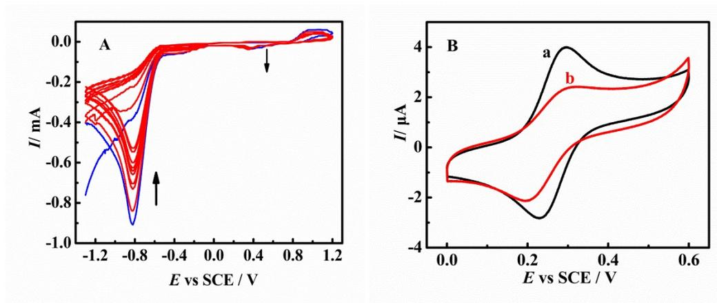
**Fig. S1** (A) Continuous CVs at  $0.1 \text{ V s}^{-1}$  for the electropolymerization of P(NIPAM-*co*-APBA) films at Au electrodes in the precursor solution. (B) CVs of  $0.5 \text{ mM}$  FCA at  $0.1 \text{ V s}^{-1}$  in pH 9.0 buffers at  $37 \text{ }^\circ\text{C}$  at (a) bare Au electrodes and (b) P(NIPAM-*co*-APBA) film electrodes.
