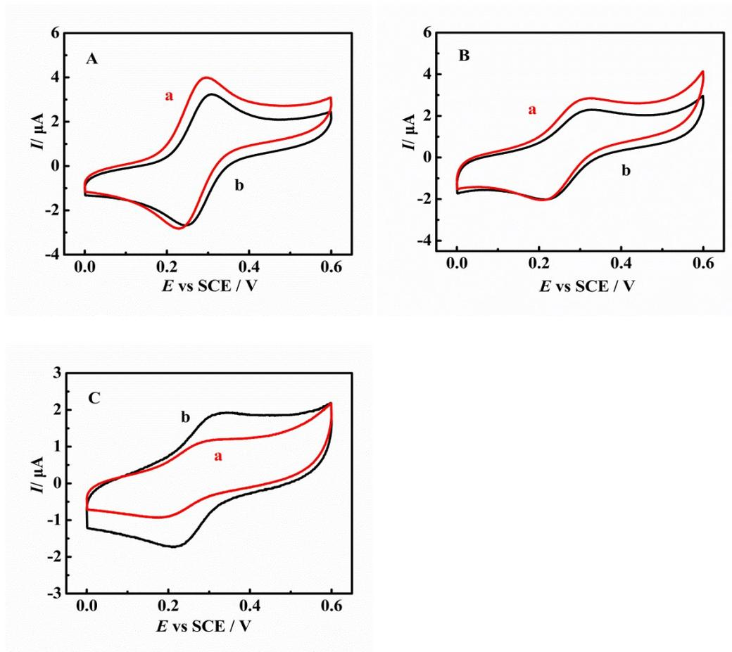
**Fig. S3** CVs of 0.5 mM FCA at  $0.1 \text{ V s}^{-1}$  at (A) bare Au electrodes, (B) PAPBA film electrodes and (C) PNIPAM film electrodes in pH 9.0 buffers at (a) 37 and (b) 20 °C, respectively.
